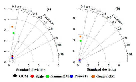
**Figure 9.** Taylor diagram shows bias correction methods' performance to downscale EC-Earth minimum temperature during (a) calibration; (b) validation periods.
