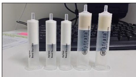
Figure 3-6: SPE pre-packed cartridges.
