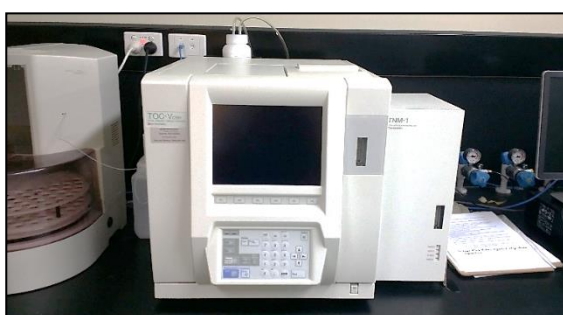
Figure 2-7: Total Organic Carbon Analyser (SHIMADZU TOC-V CSH) in USQ Water Lab.
