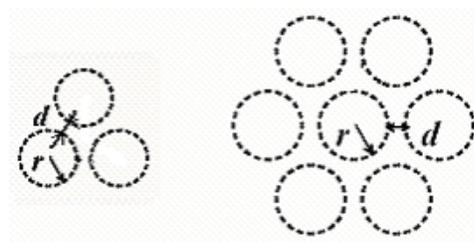
Figure 2 Schematic of the cross-section of three and seven CNT bundles.
