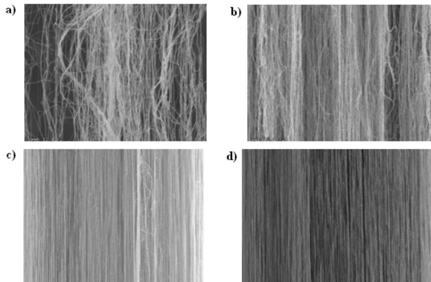
Figure 8. SEM image showing the microstructure of the bundles in webs; (a) web image using the previous process; b) web microstructure using the modified process; (c) web image under high tension between two initial rods (1) & (2) on the CERS (see Figure 6.a) and (d) web image under tension between two initial rods (1) & (2) with heat treatment.
