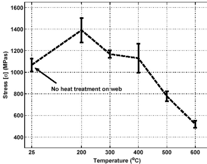
Figure15 Tensile strength of yarn samples plotted against the temperature of heat treatment on the web before going through the CERS (the dotted line represents the average values of tensile strength). The ambient temperature of the laboratory is 25°C.
