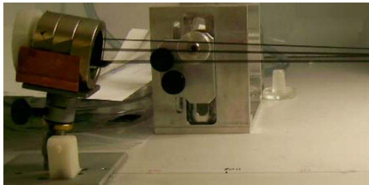
Figure 12 CNT Multi-web spinning using the modified process.
