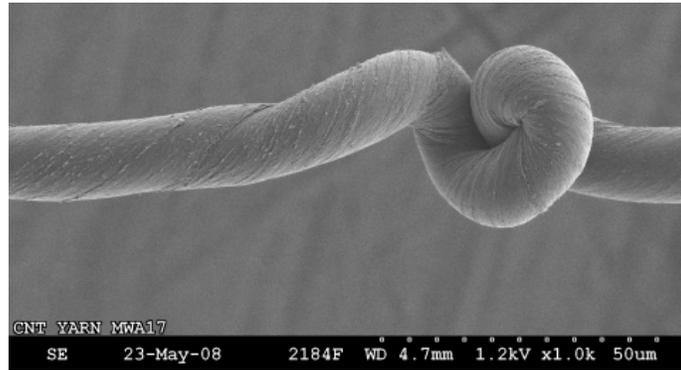
Figure 10. Micrograph of highly twisted yarn with densification: a snarl of yarn.
