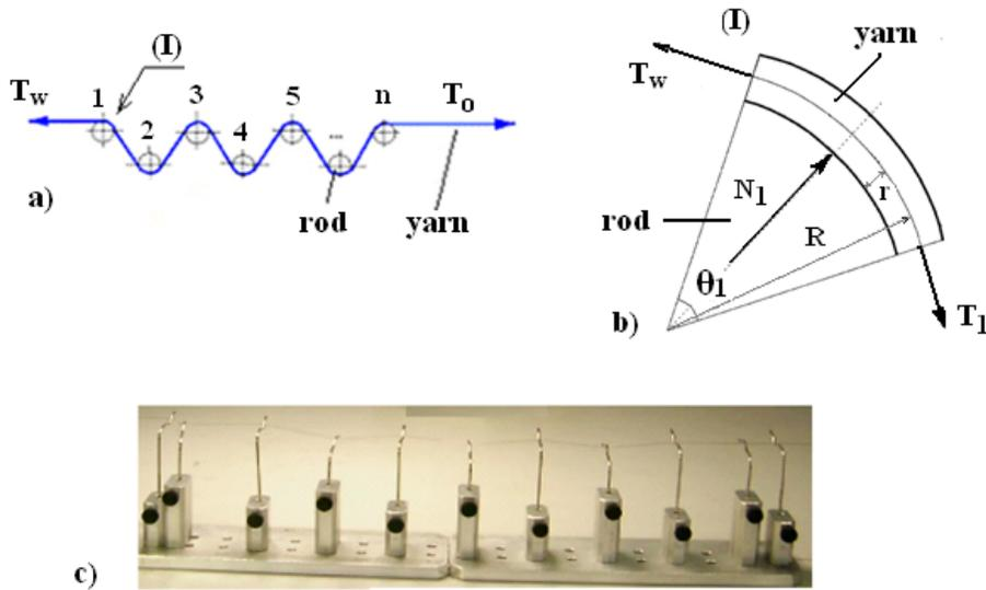
Figure 6.a) A schematic of the tensioning/drafting system using a capstan effect rod system (CERS); b) the change of tension and radial pressure in a yarn as it passes around a rod (first rod) and c) a photo of the experimental CERS.  $R$  and  $r$  are the rod and yarn diameters, respectively.
