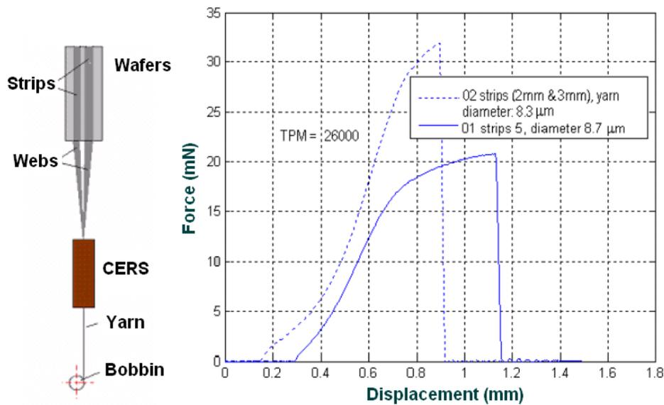
Figure. 13 Force-displacement curves of two typical samples of CNT yarn. The solid line is from one strip of 5mm and the dotted line is from two strips of 2mm and 3mm, respectively.
