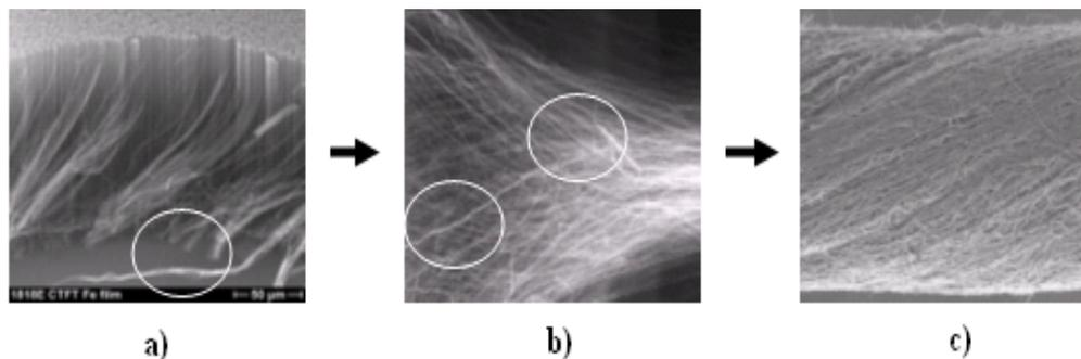
Figure1. The structure of the successive stages of the CNT spinning process: a) CNT forest structure; b) web structure and c) yarn structure. The middle picture
