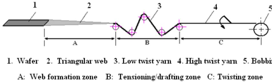
Figure 4: The schematic of modified CNT yarn spinning.
