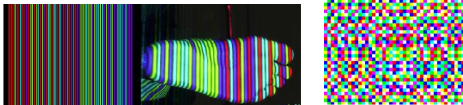
Figure 2.12: Projected Structured Light patterns. Left: Coloured stripe pattern (Thabet et al., 2014) and right: random speckled pattern (Chen et al., 2008).
