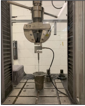
Figure 5. Experimental setup for static yield strength measurement.
