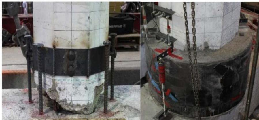
a) Steel collar and anchored steel
