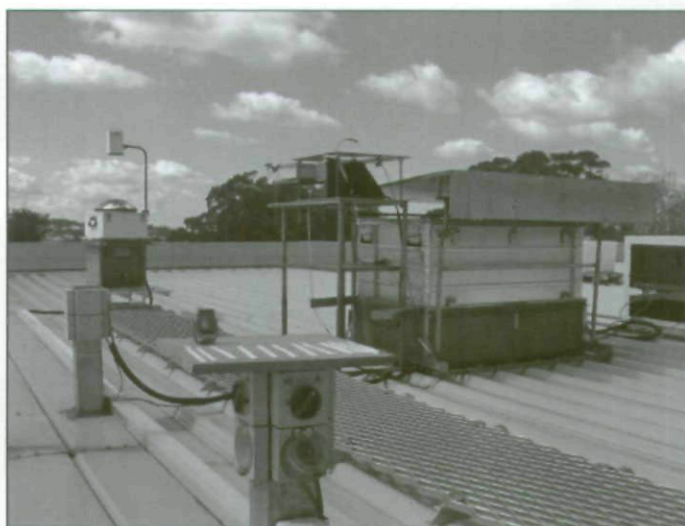
Figure 1. Dosimeter strips exposed on a horizontal plane at the University of Southern Queensland Toowoomba campus atmospheric research station. The handheld UV irradiance meter is the small device near the paper strips. In the background is the UV spectroradiometer and full sky monitor.
