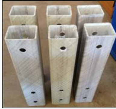
Figure 2: Vertical components of pultruded GFRP T-joint.
