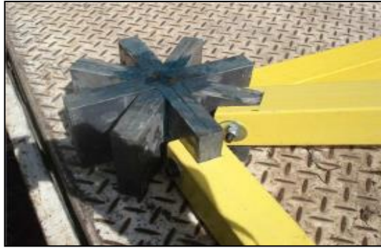
Figure 2.12. Pultruded GFRP novel connector for space truss (Bai and Yang, 2013)
