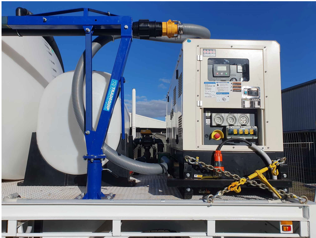
Figure 4: Autofill crane/boom arm, generator, and electronic valve V3 visible in back between generator and rinse tank
