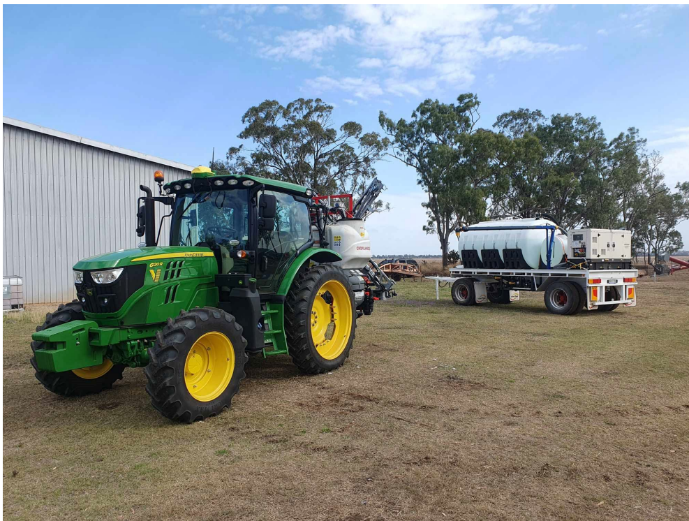
Figure 1: UniSQ John Deere 6120R with croplands section sprayer implement and IPF autofill nurse tank trailer
