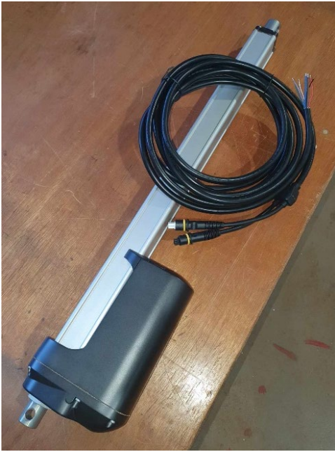
Figure 13: Linak LA36 linear actuator with 5m cable
