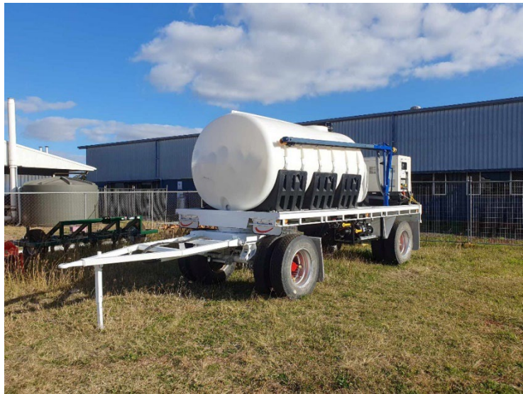
Figure 2: IPF autofill nurse tank trailer with fitted boom arm and 3-phase generator
