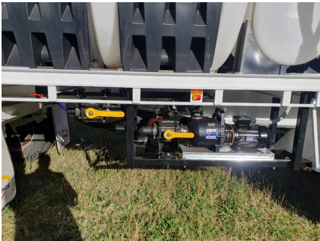
Figure 3: Autofill nurse trailer 3-phase pump and valves V1, V2
