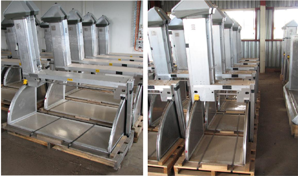
Fig 3.11 Replacement of new gates in different sizes instead of drop board checks and Detheridge wheels
