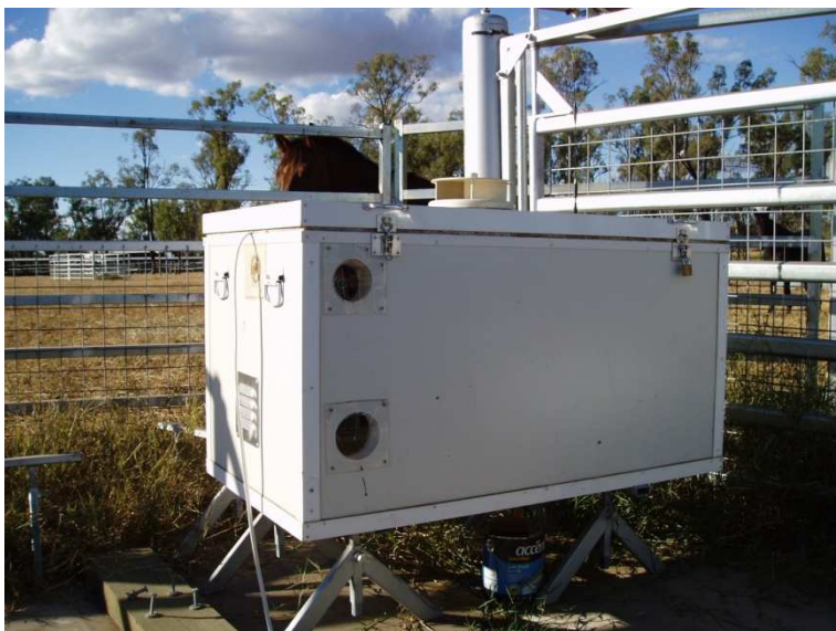
Figure 62 Insulated boxes that were used to house the prototype animal identification system
