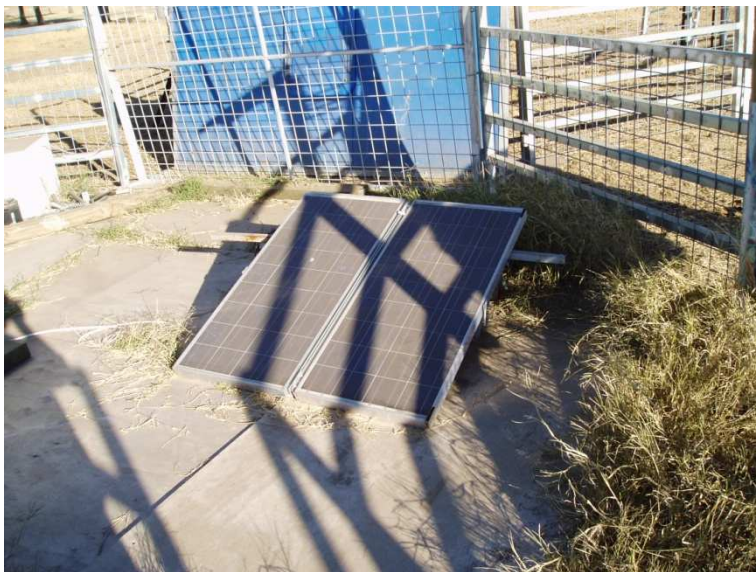
Figure 61 60W solar panels used to supply the laptop and air compressor
