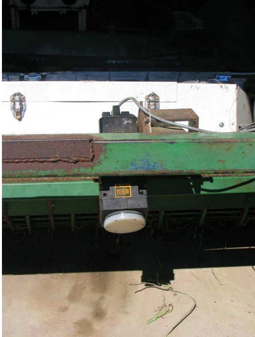
Figure 31 Ground speed radar mounted on the macadamia nut harvester
