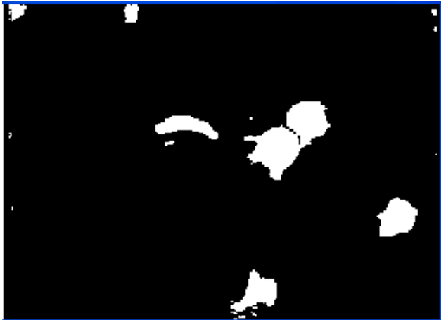
Figure 37 An example of virtual search space. The black pixels have been identified as the background, the white as non-background
