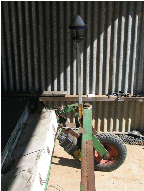
Figure 30 GPS antenna and radar mounted on the macadamia nut harvester
