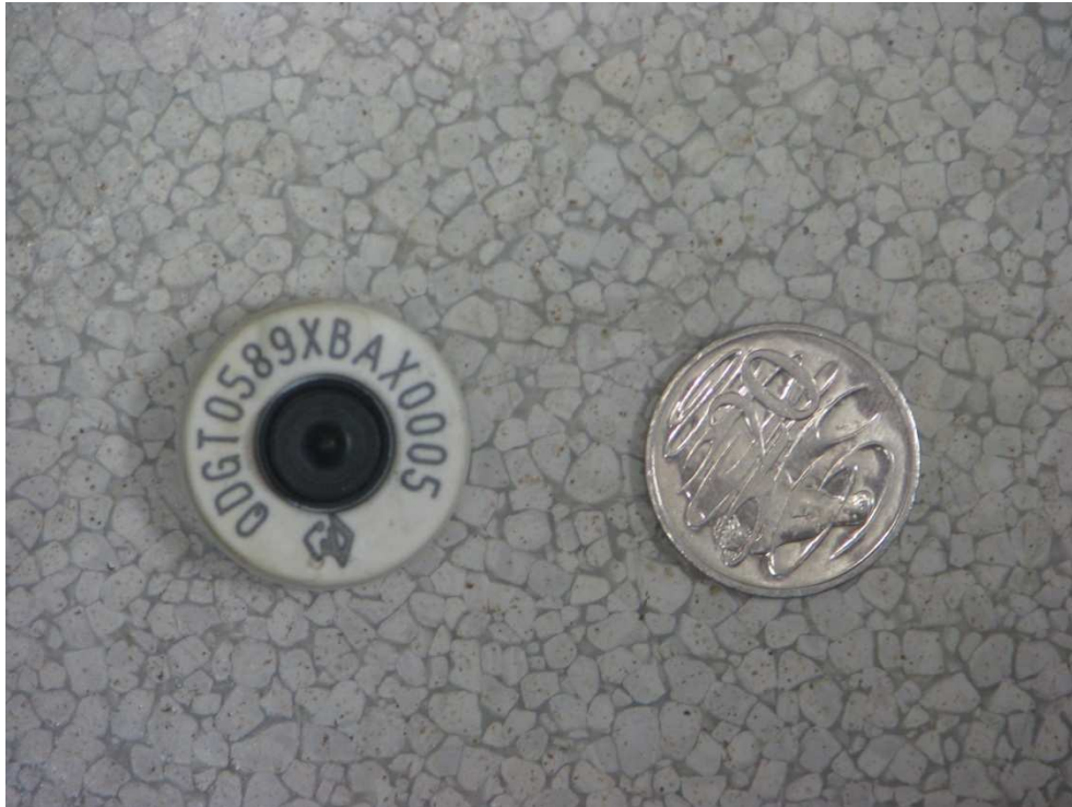
Figure 57 Standard RFID cattle ear tag device (25mm diameter) in comparison to a 20c piece
