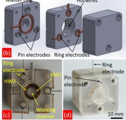
**Figure 1.** Present point-to-ring corona based gyroscope: (a) Schematic design, (b) 3D sketch and (c, d) experimental prototype.
