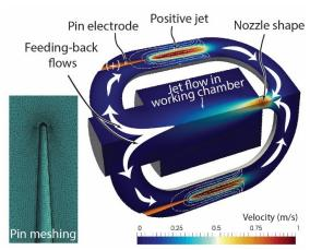
**Figure 3:** Simulation showing flows circulating inside the sensor using OpenFOAM.
