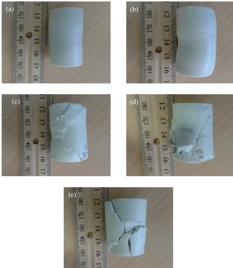
Figure 3.13: Representative specimens of failure mechanism sequence in syntactic foam (a) SCFT-01 and (b) SCFT-02 have barrel shape failure mode (c) SCFT-03 (d) SCFT-04 and SCFT-05 have spalling of syntactic foam
