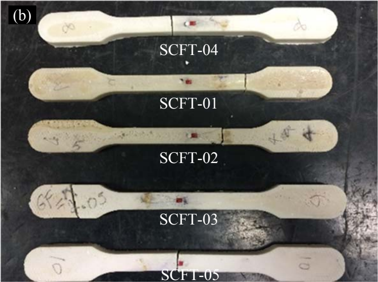
Figure 6.18: (a) Matrix particle debonding of tensile specimen (b) Representative of the tensile fractured specimens
