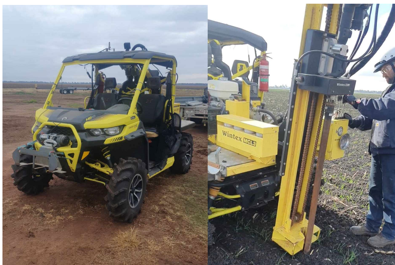
Figure 6. Example of vehicle-based soil testing with a Wintex MCL3.
