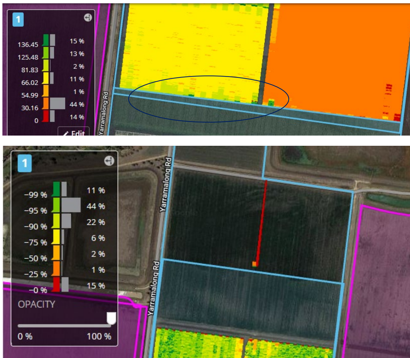
Figure 12. As-applied map showing areas of high initial flow rate (circled in top), and as-applied quality map showing section off the top of the Figure 11 map.
