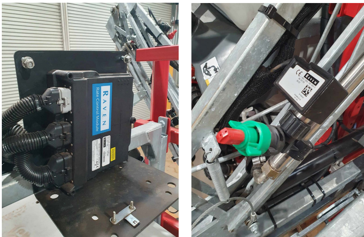
Figure 2. Raven rate control module (left) and Hawkeye 2 nozzle controller (right)
