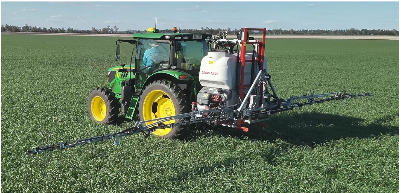
Figure 1. Croplands 3-section sprayer mounted on John Deere 4066R
