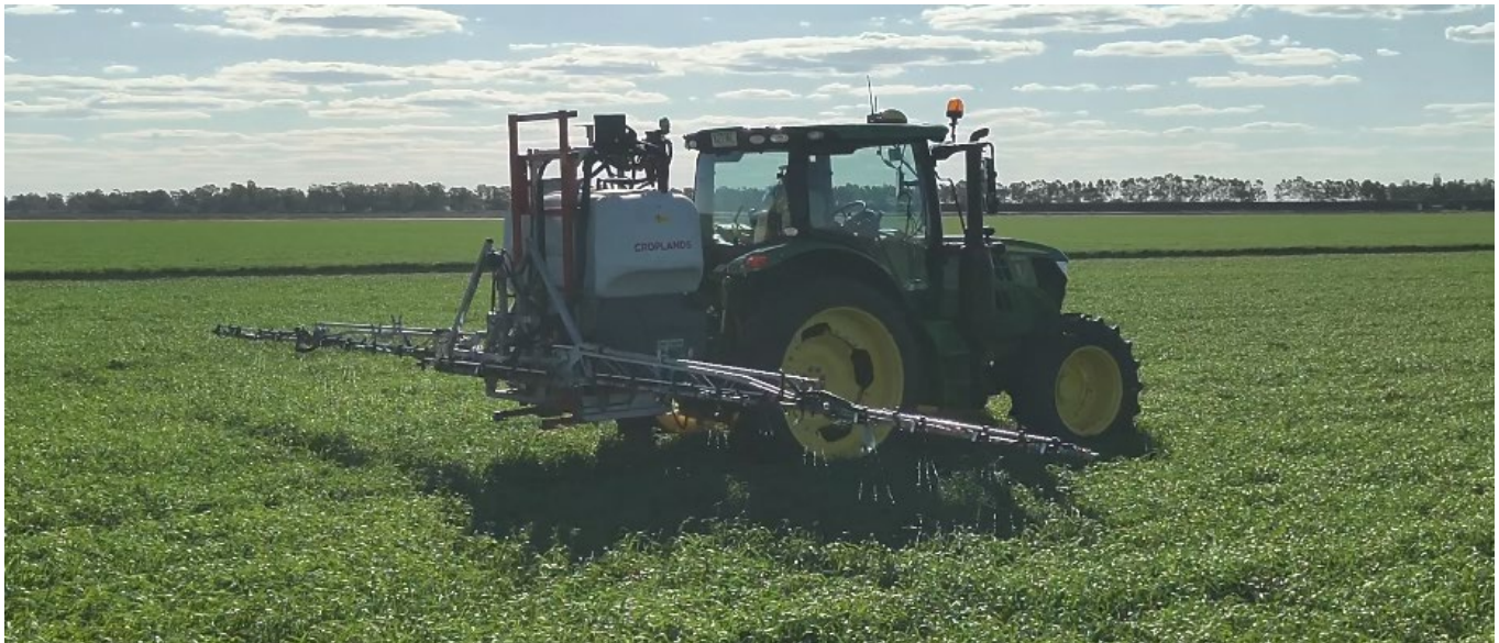
Figure 10. Sprayer applying Easy-N to a wheat field. The streams can be seen in front of the tractor wheel.
