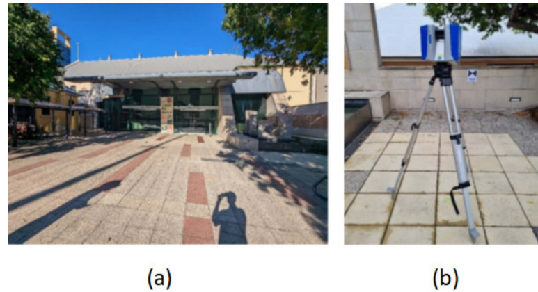
Figure 5. Scanning site and static scanner: (a) area of interest and (b) TLS equipment Z+F 5016 static, operating within the outdoor area.
