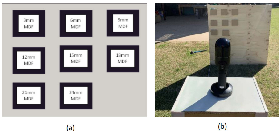
Figure 7. (a) Edge detection board and (b) edge detection board with the SLAM scanner.
