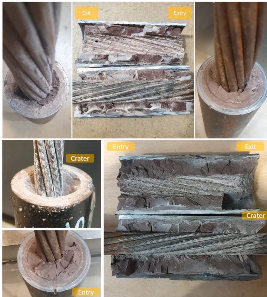
Fig. 6. Top: Goliath cable after the test in grout – before and after cutting – Bottom: Indented Superstrand cable after the test.
