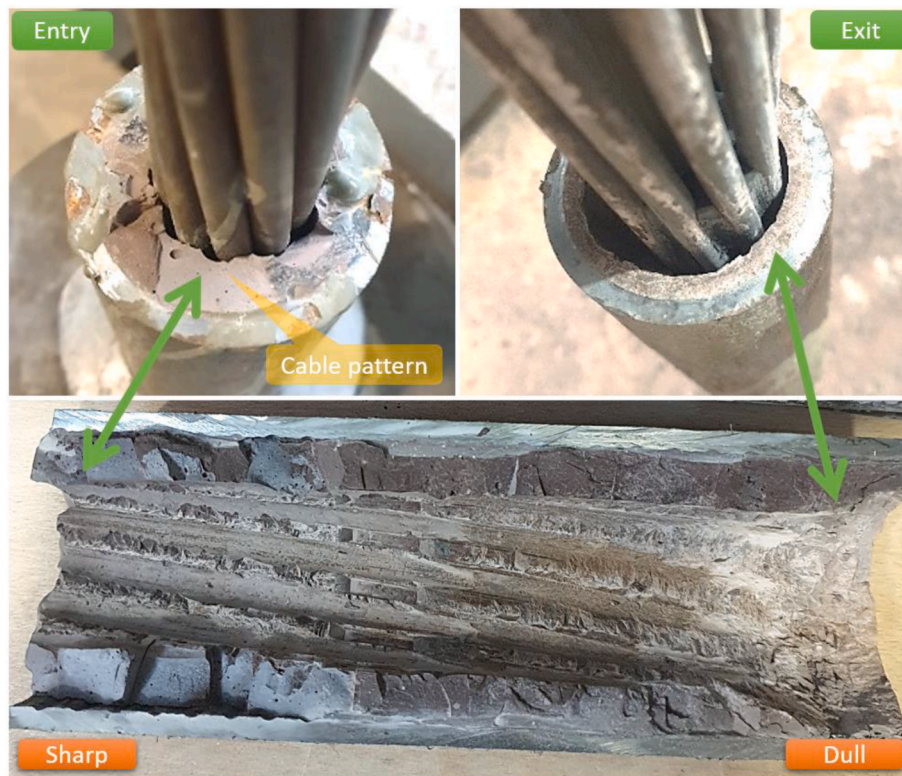
Fig. 8. 10 strand cable after the test – mismatched cable pattern in entry point and scraped exit point.
