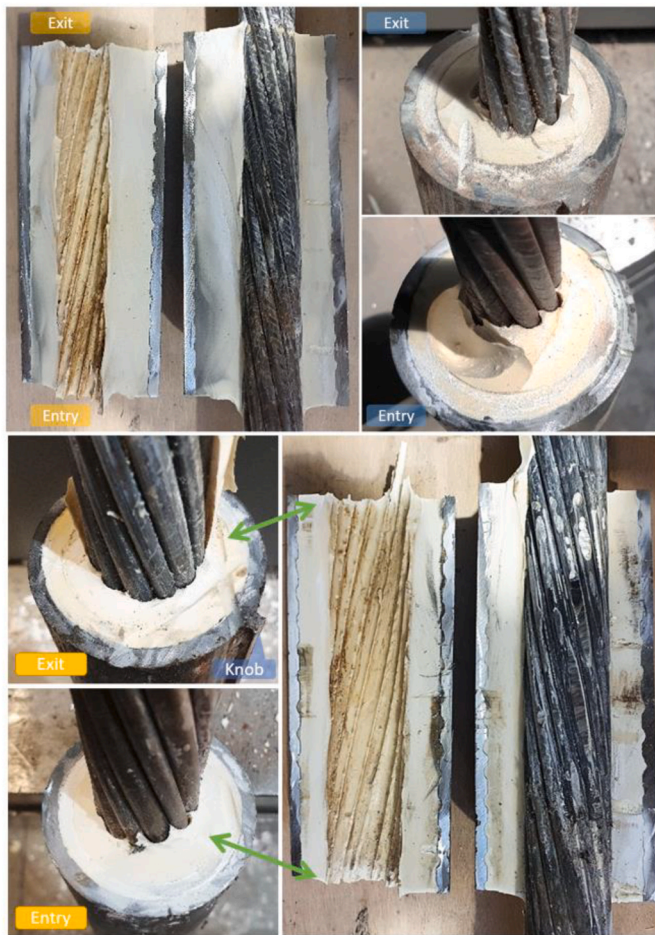
Fig. 10. Top: Indented Superstrand sample in resin – Bottom: Goliath cable in resin after the test.
