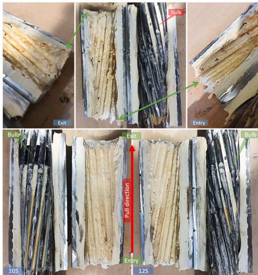
Fig. 11. Top: The entry and exit point conditions after the 9S cable test in resin sleeve pull out – Bottom: The bulb location after the 10S and 12S cables in resin sleeve pull out.
