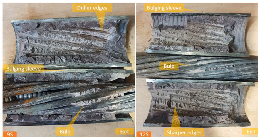
Fig. 7. Open 9 and 12 strand cables after the test.
