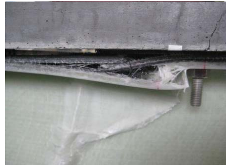
HFRP flange delamination failure (SA-135-50)
