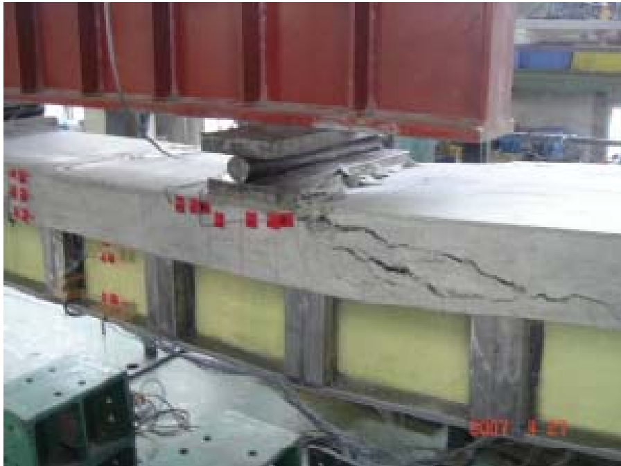
Compression failure of NSC slab
