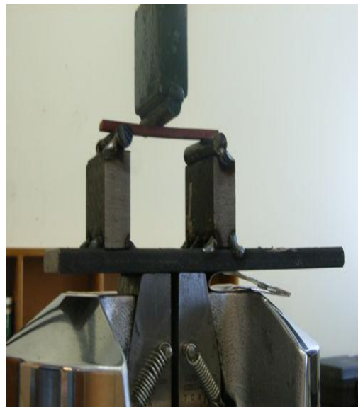
Figure 2: Three-point bending test on flexural specimen
