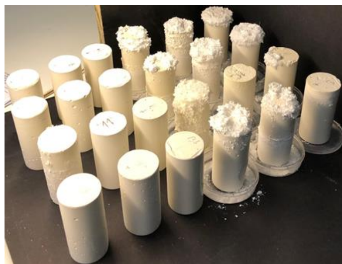
Fig. 2-63 Alkali-activated metakaolin specimens exposed to efflorescence condition
