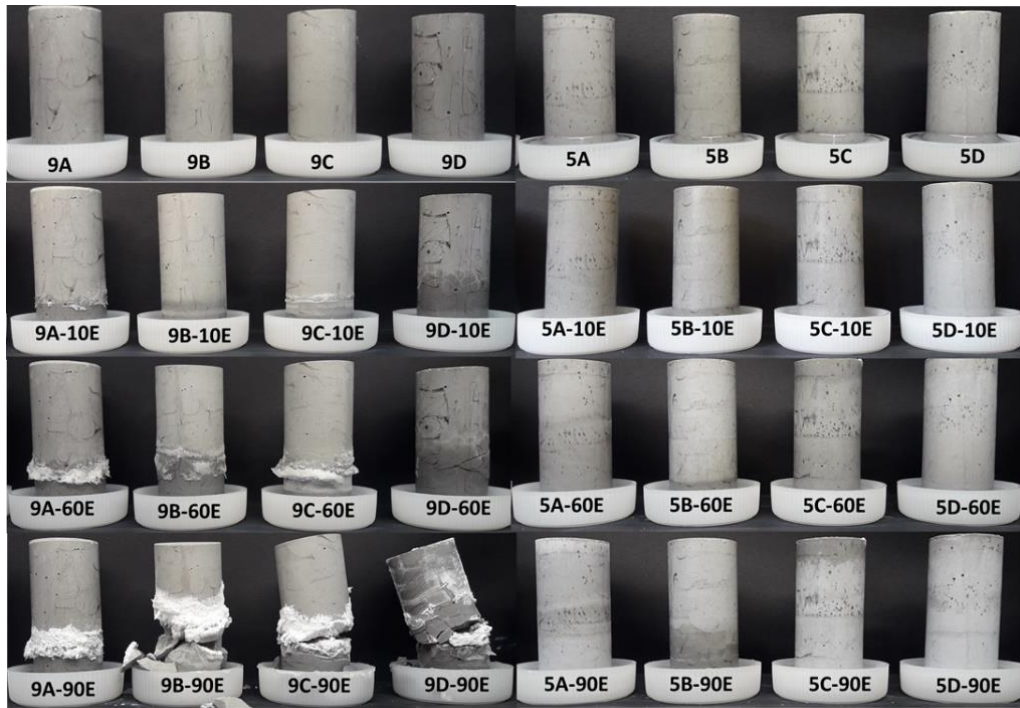
Fig. 6-3 Cylindrical binder specimens before and after 90 days of efflorescence exposure
