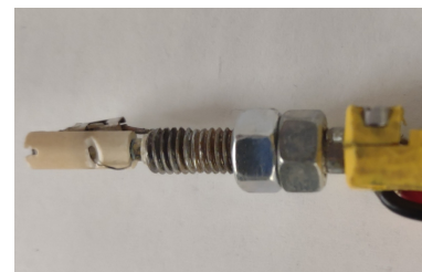
Figure 3. Details of the thermocouple used in the present work.
