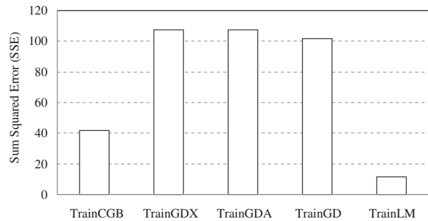
Fig. 8 Comparison of performance after 300 epochs with different training functions
