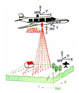
Figure 1. A Typical LiDAR System (Gross, 2003)
