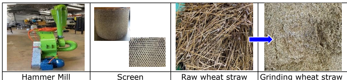
Figure 3.2: Hammer mill and ground wheat straw
