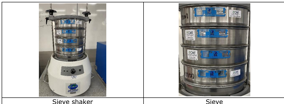
Figure 3.3: Sieve analysis of wheat straw and saw dust
