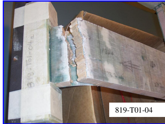
Figure 4.4 T01-04 - Failure mode
