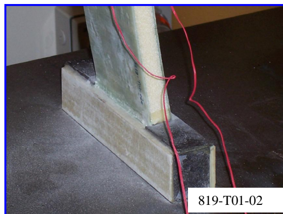
Figure 4.3 T01-02 - Failure mode
