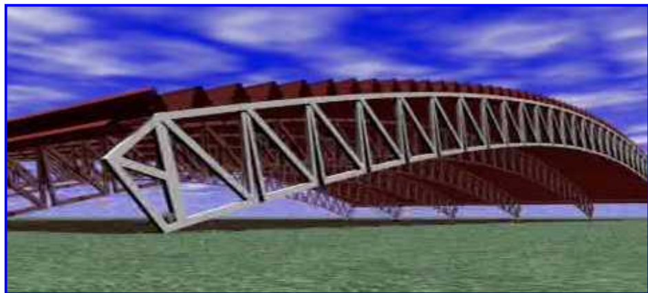
Figure 1.4 Stressing the frames during erection stage
