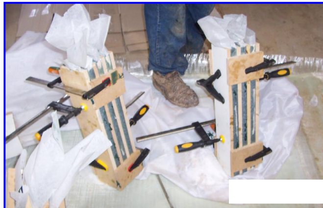
Figure 4.12 Gluing skins to the core for single core columns
