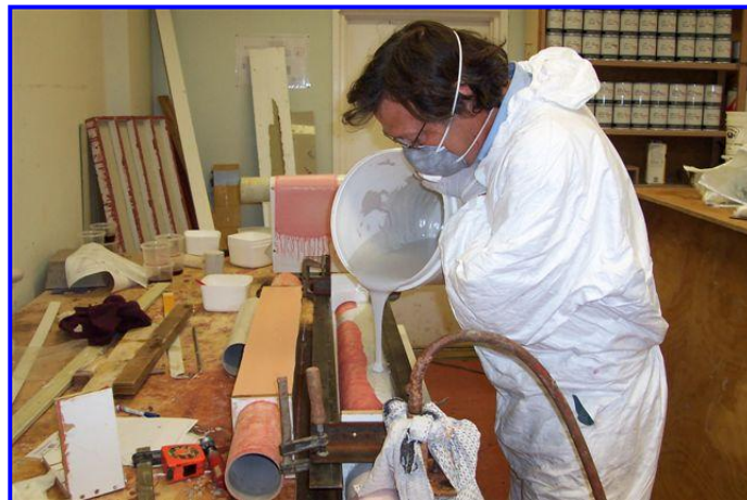
Figure 3.2 P109 – Casting PFR on the chord members
