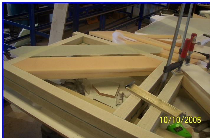
Figure 3.11 P309 - Assembling the first two frames
