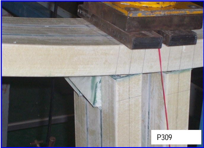
Figure 3.27 P309 - Sway after reaching ultimate capacity
