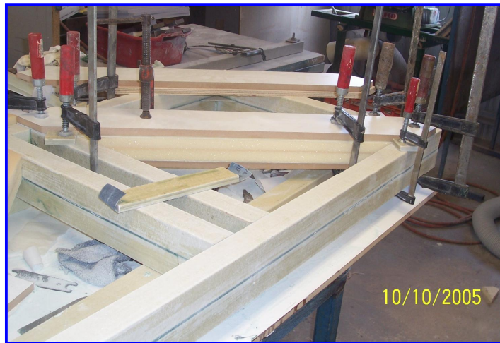
Figure 3.12 P309 - Assembling of diagonals
