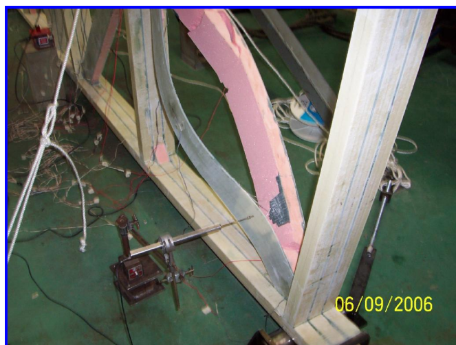
Figure D.17 P819 - Failure due to shear buckling
