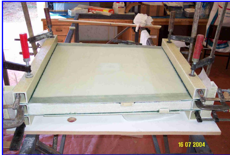
Figure 5.2 P509 – Panel during assembly
