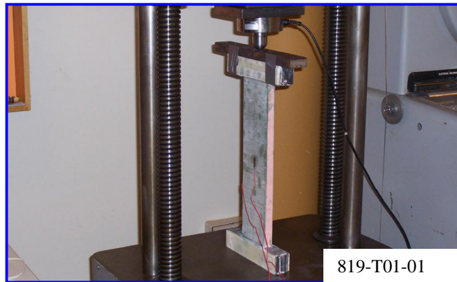
Figure 4.2 Prototype test layout of T01 columns
