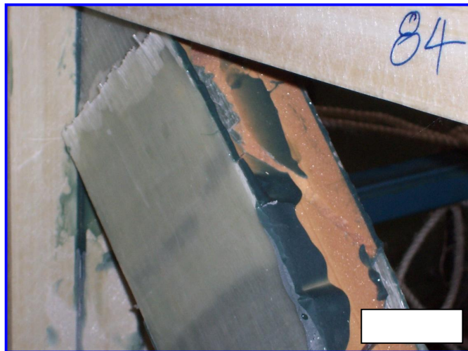
Figure 4.36 P409 - Failure at the upper corner
