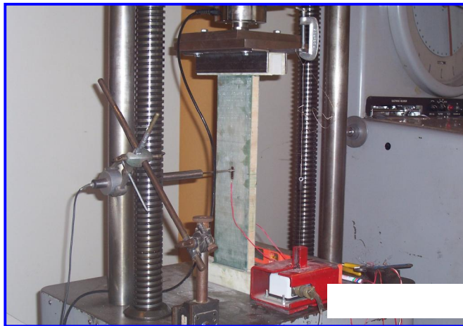
Figure 4.14 T02 - Columns test setup
