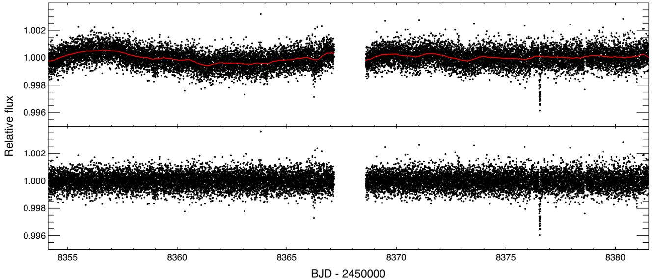
**Figure 1.** *TESS* data of TOI-222. The top panel shows the uncorrected data in black with the 10-h boxcar applied to correct for stellar and instrumental systematics in red. The bottom panel shows the corrected *TESS* data.
