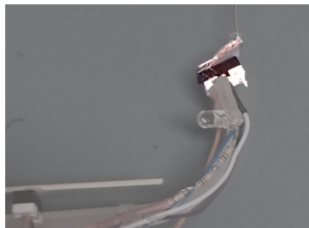
Figure B.4. The touch sensor switch, attached to right scoop arm.
