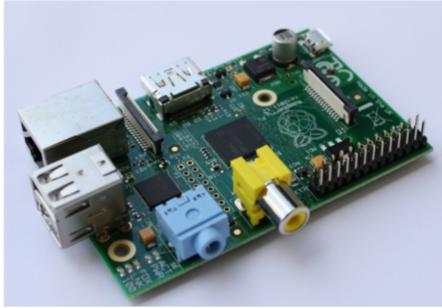
Figure B.2. The Raspberry Pi model B (revision 2) single board computer – the primary computer in all physical agents. From the Raspberry Pi Foundation.
