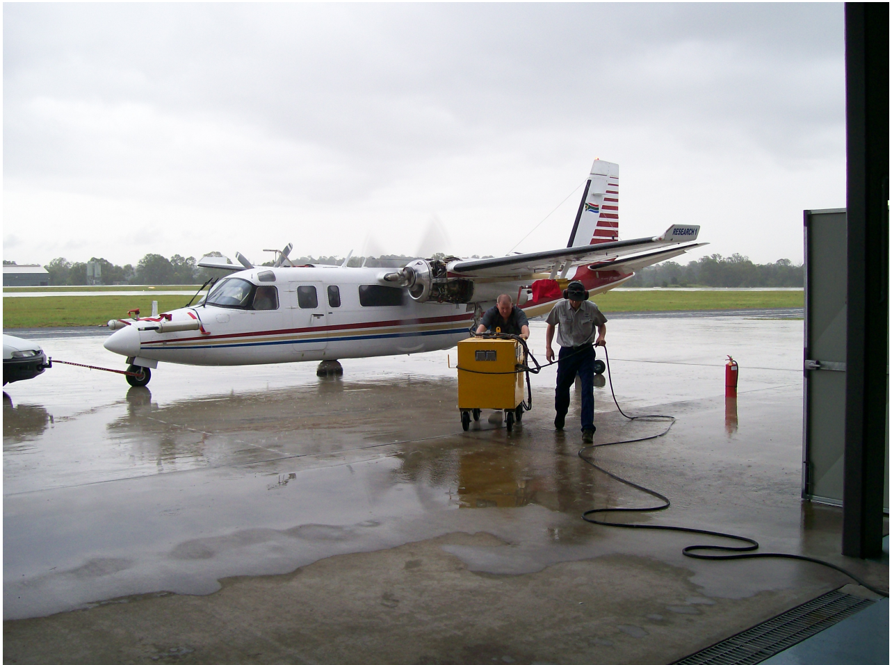
Figure 1 SAWS Aerocommander 690A (ZS-JRA) carrying out ground tests following a successful full turboprop engine replacement which took less than two weeks to complete. Engineer : Harry McGarry. Pilots :- Ret Orsmond, Hans Krugar, Gary Wiggins and John Hingst.
