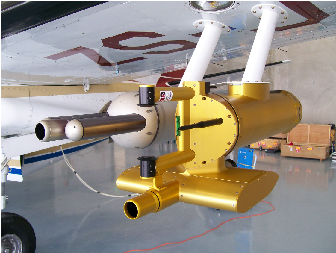
Figure 4 CAPS probe (on right) incorporating four cloud physics measuring instruments including - Cloud Imaging Probe (CIP), Cloud and Aerosol Spectrometer (CAS), Liquid Water Content (LWC) hot wire instrument in addition to a pitot pressure tube
