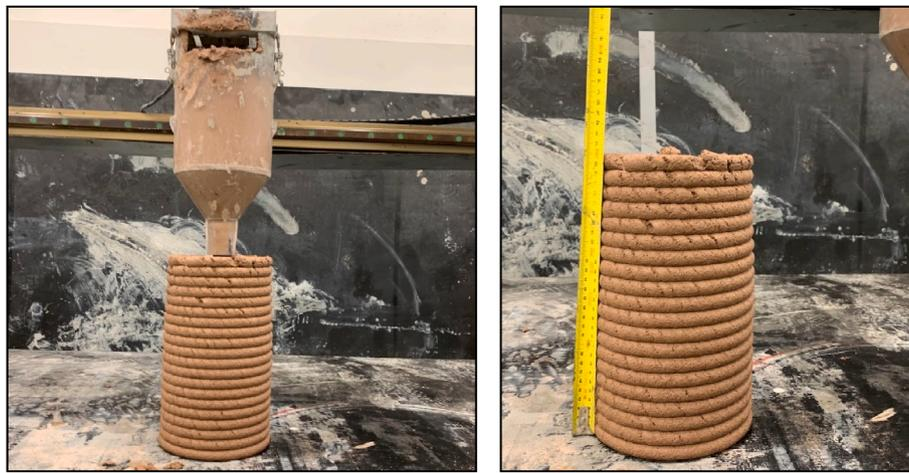
Fig. 9. 3D printed structures using optimum mix (M<sub>3</sub>).
