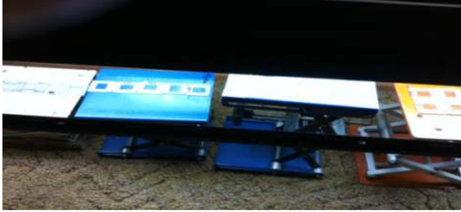
Figure 11 The fluorescent tube exposing dosimeters at different distances of 5 cm, 10 cm, 15 cm and 20 cm
