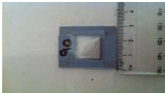
Figure 2 Dosimeter with polysulphone and phenothiazine films and a Llumar filter
