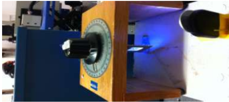
Figure 10 A solar simulator exposing dosimeters at different angles
