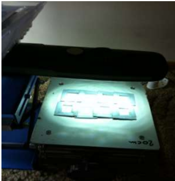
Figure 3 LED light exposure for eight dosimeters to determine the dose response
