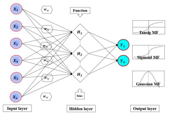
**Figure 3.** Typical ANN architecture for SSL modeling where *w*: weight and bias are justified by the training process. Most common transfer functions are sigmoid, Gaussian and tangent sigmoid (i.e. tansig).
