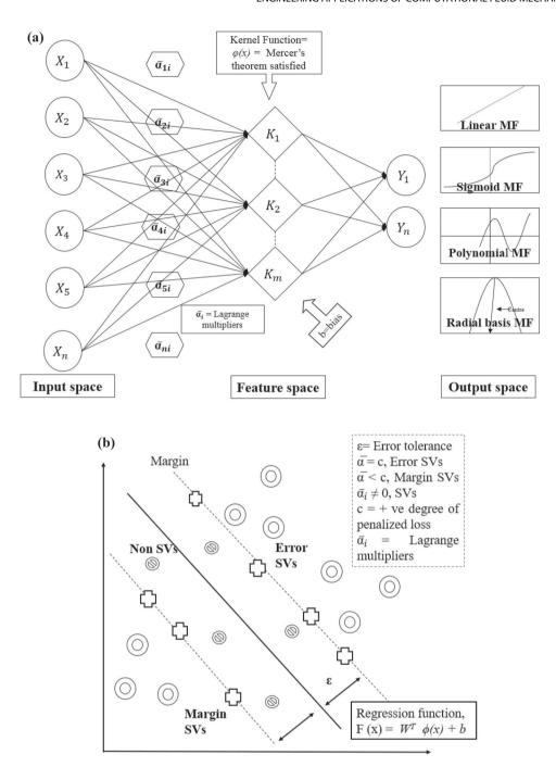
**Figure 4.** (a) Typical SVM architecture for SSL modeling where  $\overline{\alpha} =$  weight and b = bias. Most common transfer functions are linear, polynomial, radial basis, and sigmoidal, K = support vector, m = number of support vectors,  $\varphi(x) =$  non-linear function. (b). Non-linear SVR vapnik's  $\epsilon$ -insensitivity loss function.
