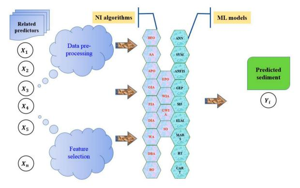
Figure 12. Proposed scheme of hybrid predictive models based on the hybridization of nature inspired optimization algorithms with standard artificial intelligence models.
