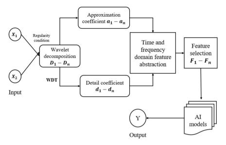
Figure 7. Schematic diagram of hybrid wavelet-Al model: regularity condition with order N decides the choice of wavelet. Wavelet denoising (WDT) is applied to adjust detail coefficient. X1 and X2 = Input variables, D1-Dn = decomposition level, Y = Output variable.
