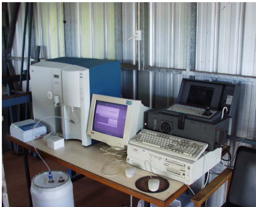
Fig 9.8 The Aromascan A32S and experimental set-up for odour sample analysing
