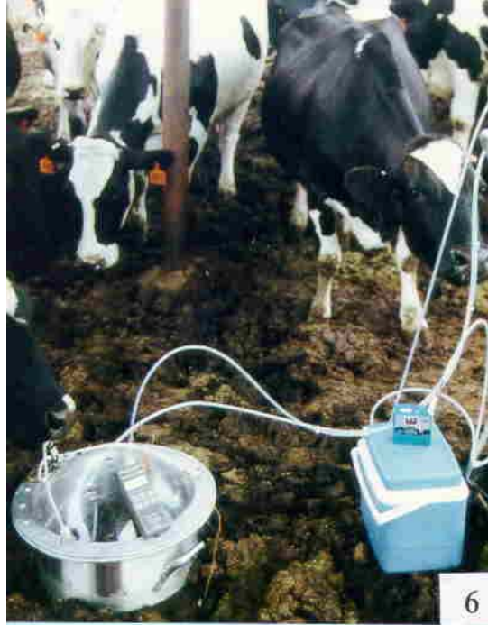
Fig 3. 2 The emission assessment using the isolation flux hood in dairy industry (reproduced from http://www.ceschmidt.com )
