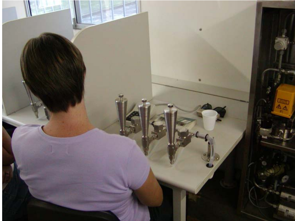
Fig 4.2 Human panellist workstation in the mobile olfactometer
