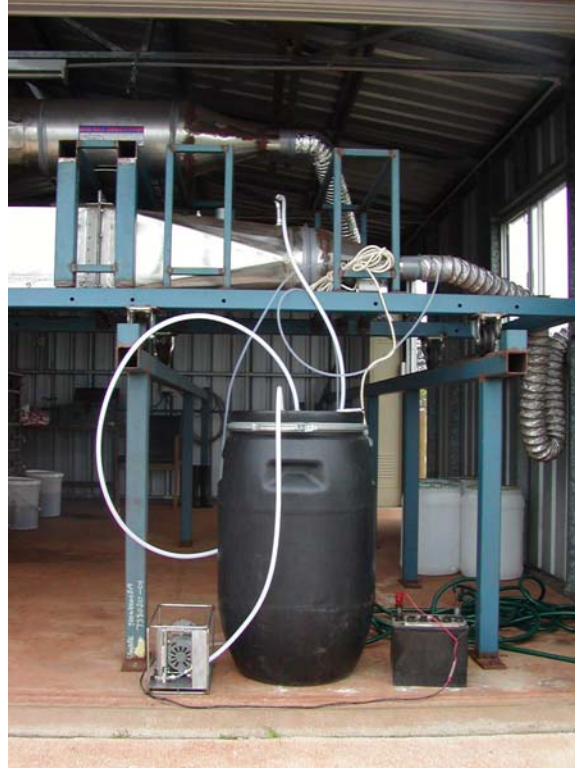
Fig 9.7 The 120L odour sample container and a diaphragm pump for olfactometry analysis
