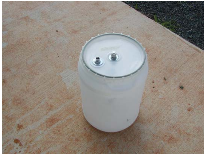
Fig 9.6 The 30L odour sample container for the AromaScan analysis
