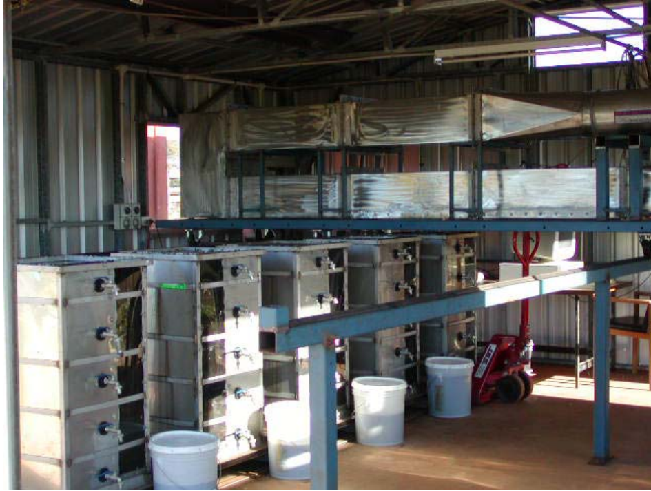
Fig 9.4 Experimental facility used to quantify effects of pond loading rates on odour emissions
