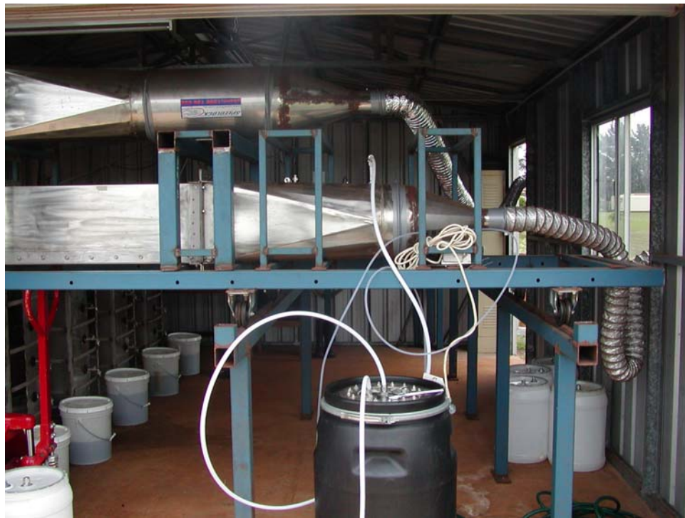
Fig 3.4 Modular designed wind tunnel with variable speed fan developed at USQ
