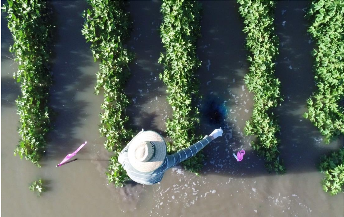
Figure 6.12 Estimating the flow rate in the furrows using UAV and food colouring technique.
