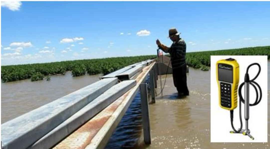
Figure 4.24 Measuring the flow rate at check gate in Field 3 (photo inset SonTek FlowTracker 2 taken from SonTek a Xylem brand website).
