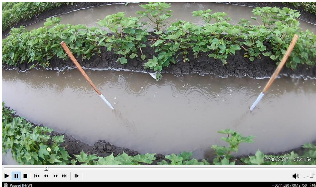
Figure 6.10 Image from a video recorded by an action camera to measure the water velocity between two stakes spaced 1 m apart.
