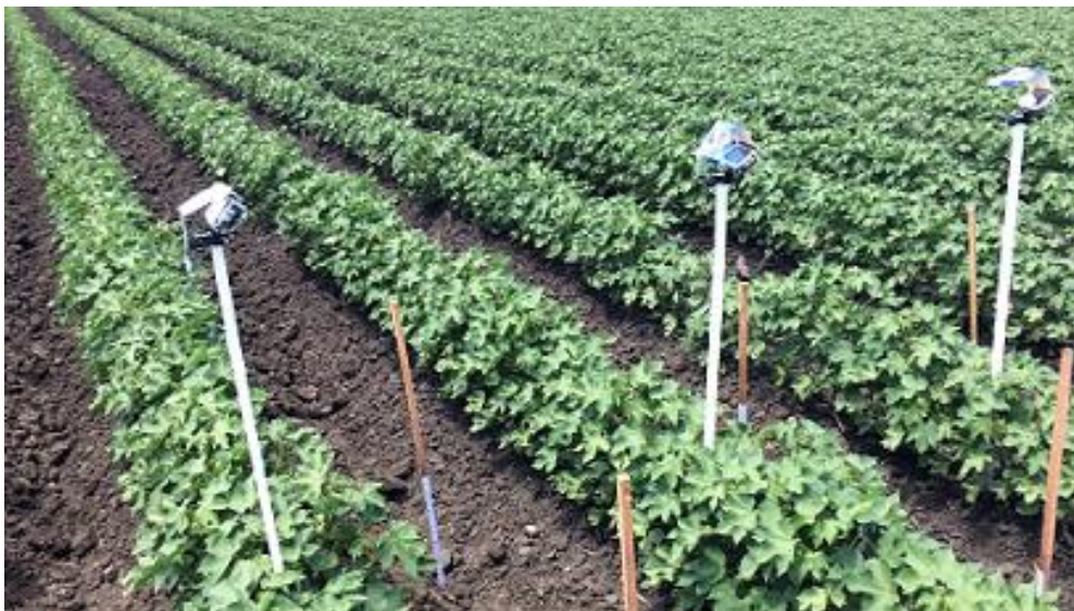
Figure 6.9 Three action cameras mounted on wooden stakes to record water velocities in three furrows at many time intervals during the irrigation event.
