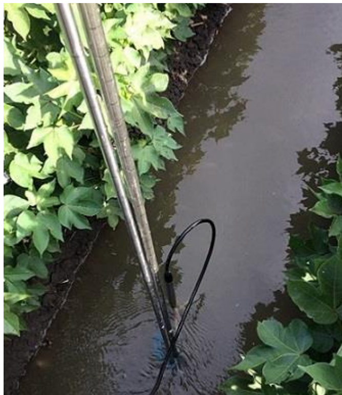
Figure 4.27 Flow rate measurement in the furrow via SonTek FlowTracker2.
