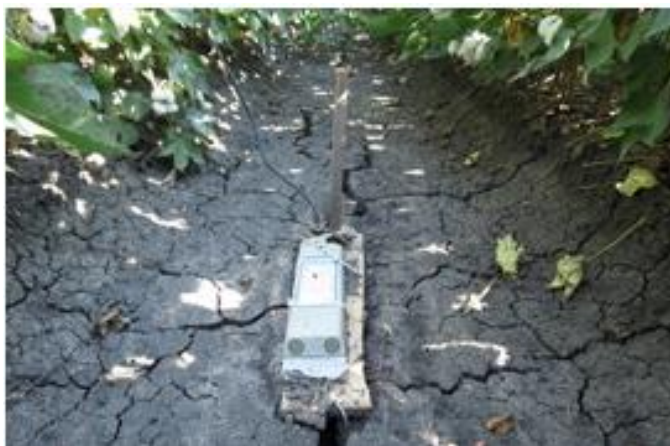
Figure 6.8 Flow measurements at the furrow scale using Starflow instruments mounted in the Furrows 4 and 6 in Borders 1 and 2 of Field 2.
