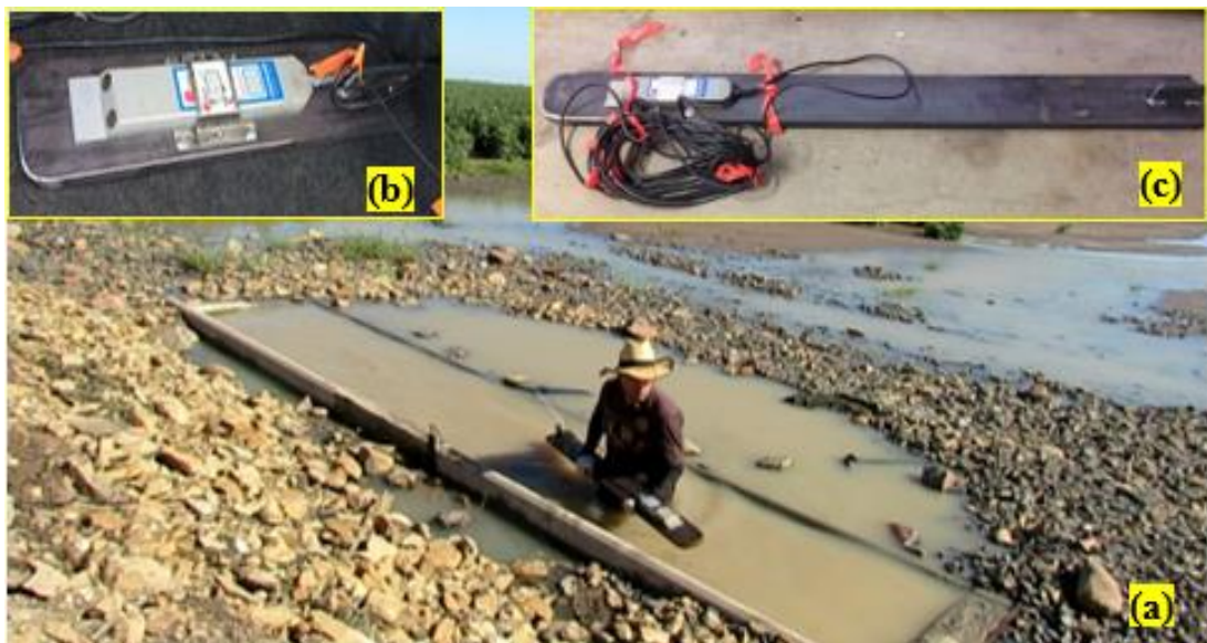
Figure 4.23 a) An attempt to mount the Starflow in the pipe of the outlet structure using a heavy piece of flat steel. B) Small piece of metal. C) Large piece of flat steel.
