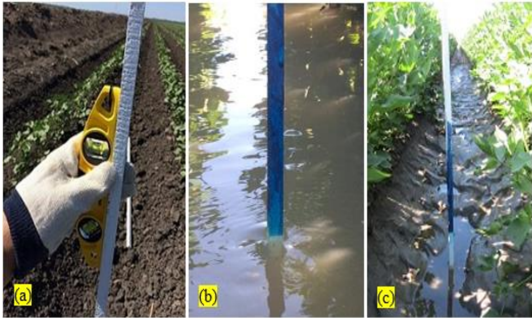
Figure 6.18 Peak water measurement via food-colouring painted stake in the furrows, showing a) insertion of the painted stake into soil using a hammer and a spirit level, b) a painted stake during an irrigation event, c) a painted stake after an irrigation event.
