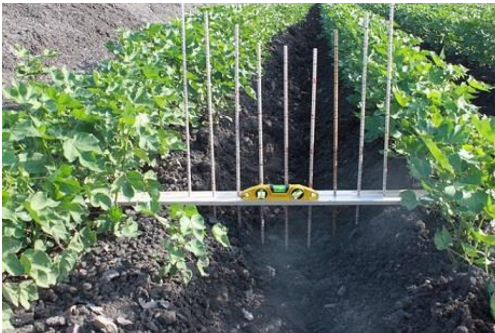
Figure 6.1 Profile meter with graduated dowels, used to measure the furrow cross sectional area.
