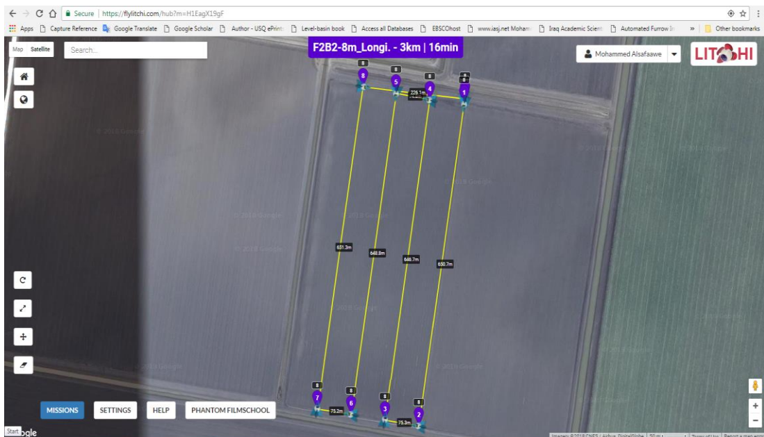
Figure 6.15 Litchi hub website with one of the flight mission with longitudinal paths in Border 2 of Field 2.
