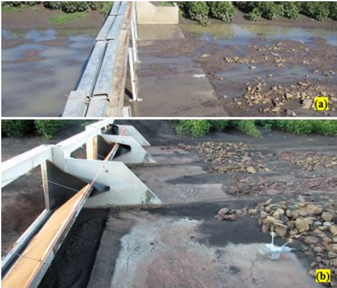
Figure 4.22 Starflow; a) Starflow mounted directly on the concrete at check gate 1, b) Starflow mounted on a bracket above the concrete to avoid being covered by deposition of eroded silt and mud at gate 2.
