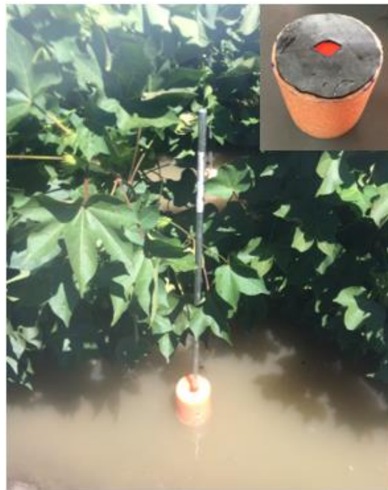
Figure 6.17 Peak water depth gauge inserted in the middle of the furrow, and a picture insert of the foam float with the rubber washer on top.
