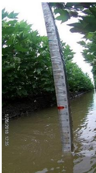
Figure 6.16 Photo taken by an action camera to measure the water depth at specific time in one furrow.
