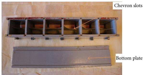
FIGURE 4: The PVC short bar test mould.
