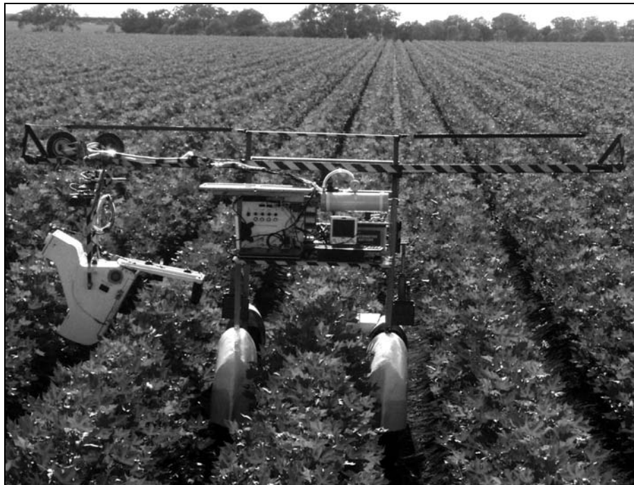
Figure 5. Automatic conveyance of camera enclosure in a cotton crop.
