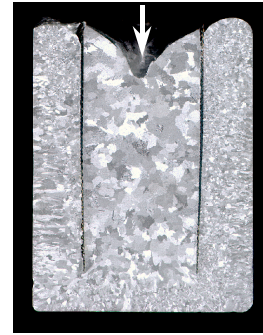
Figure 1: Etched cross-section of a cylindrical casting with a gauze barrier, showing the different grain structures generated inside and outside the gauze when internal pouring is employed.
