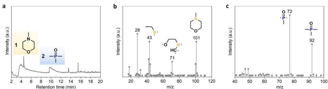
**Figure S2.** Gaseous pyrolysis products of DM-O at 550 °C. (a) Gas chromatogram, mass spectra of (b) compound 1 and (c) compound 2.
