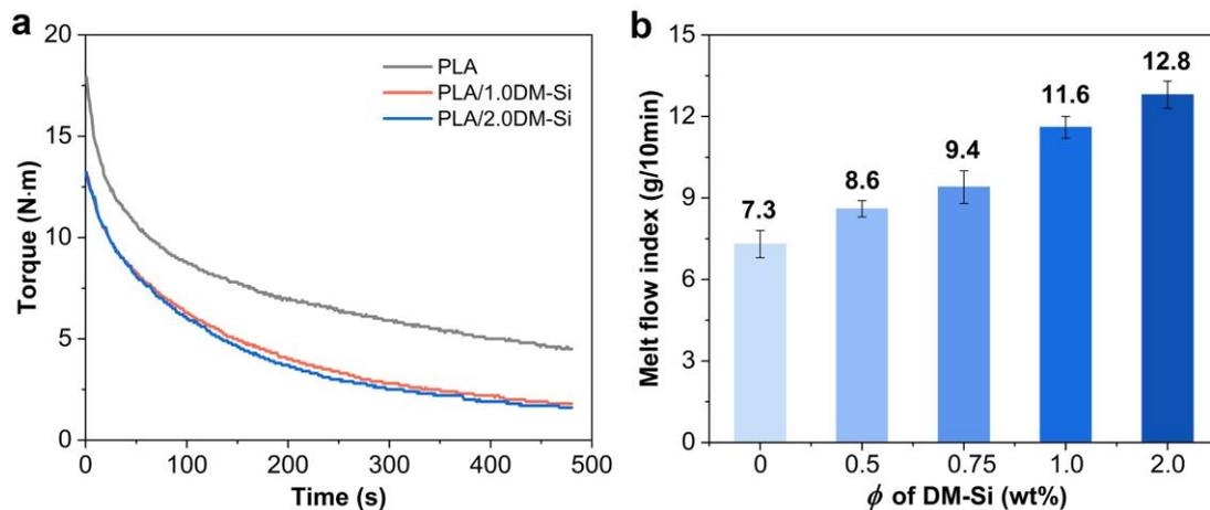
**Fig. S5.** The melt viscosity of PLA and PLA/DM-Si composites. (a) torque curves during melt blending at 180 °C, (b) melt flow index values tested under 2.16 kg loading at 180 °C.
