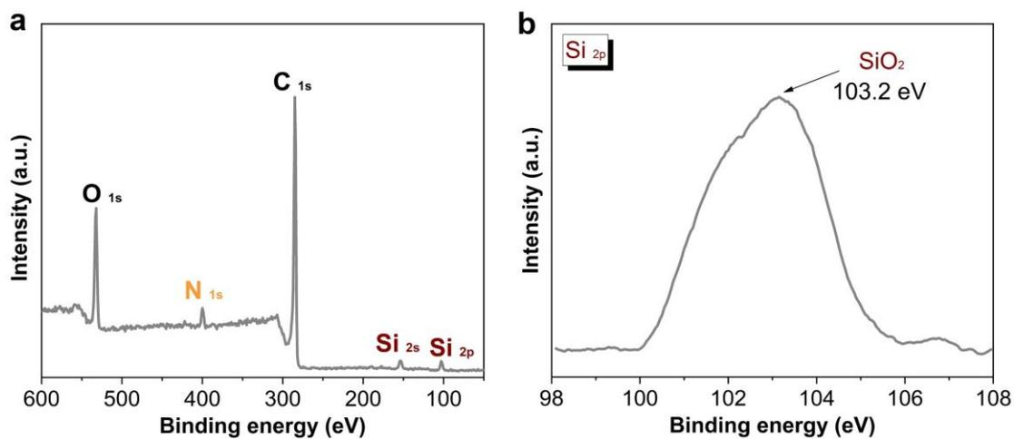
**Fig. S7.** XPS spectra of the char residue from PLA/2.0DM-Si. (a) full XPS spectrum, (b) high-resolution XPS spectra of Si 2p.
