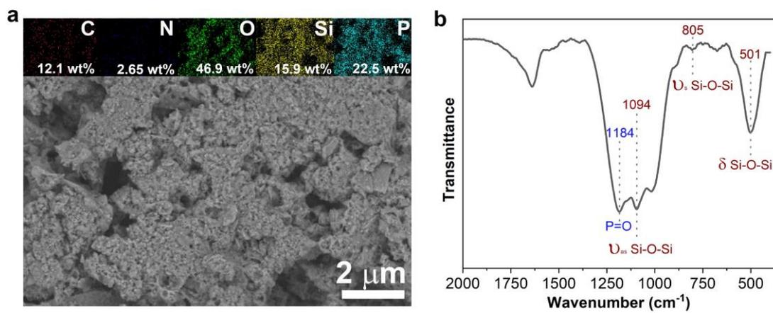
**Fig. S3.** Analysis of the DM-Si residue obtained in air atmosphere. (a) the SEM image with embedded element mapping images, (b) the FTIR spectrum.
