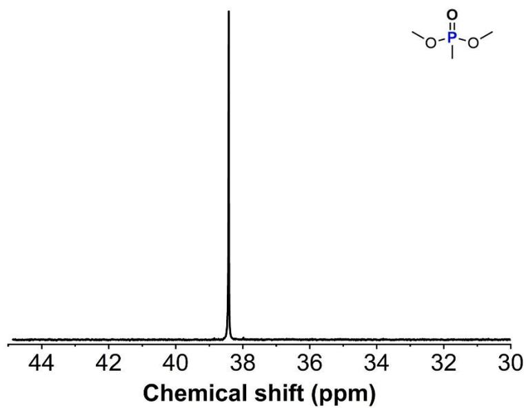
**Figure S2.** The  $^{31}\text{P}$  NMR spectrum of DMMP.
