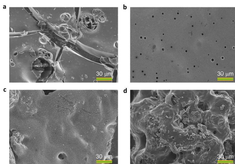
**Figure S3.** SEM images of char residue of PLA and its composites after cone
