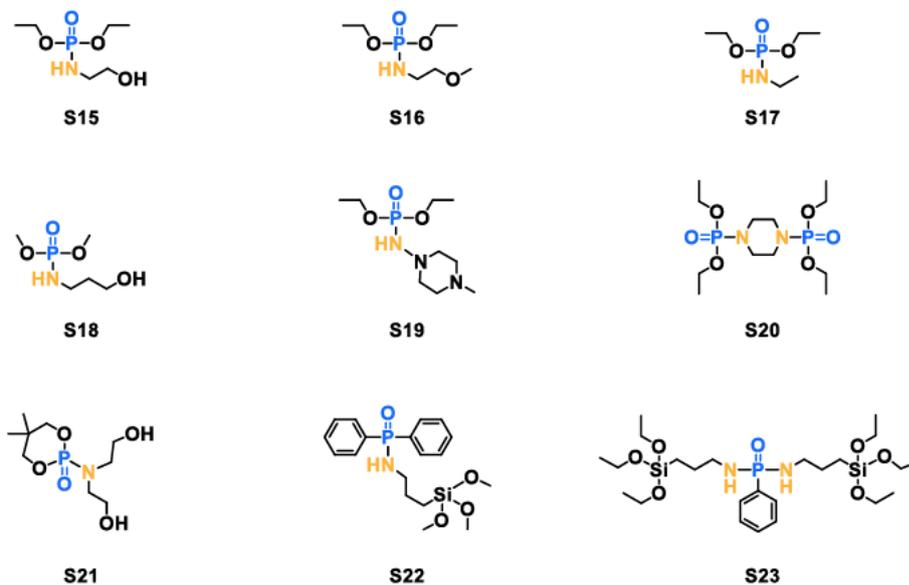
**Figure 2.4.** Chemical structures of small-molecular phosphoramidates for treating cotton fabrics.
