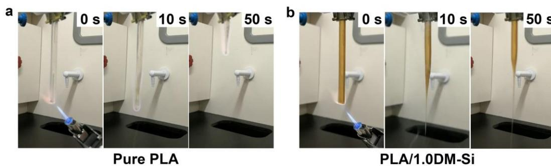
**Fig. S4.** Burning rate testing of (a) PLA and (b) PLA/1.0DM-Si.
