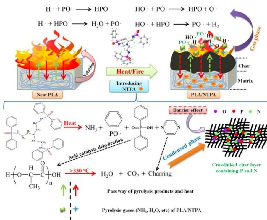
**Figure 2.2.** A typical flame-retarding mechanism of P/N synergistic (Liu et al., 2021).
