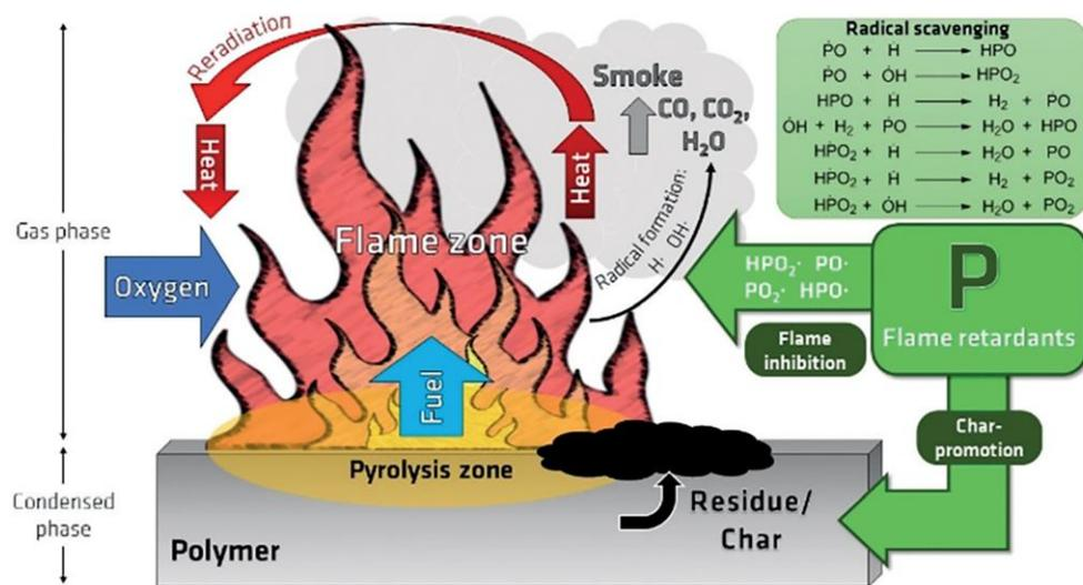
**Figure 2.1.** Flame-retarding Mechanism of phosphorus-based fire retardants (Velencoso et al., 2018).
