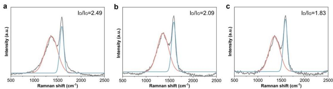
**Fig. S8.** Raman spectra of (a) PLA, (b) PLA/1.0DM-Si and (c) PLA/2.0DM-Si
