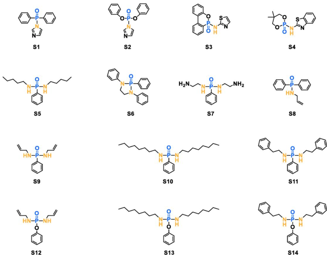
**Figure 2.3.** Chemical structures of small-molecular phosphoramidates used in Epoxy resin.
