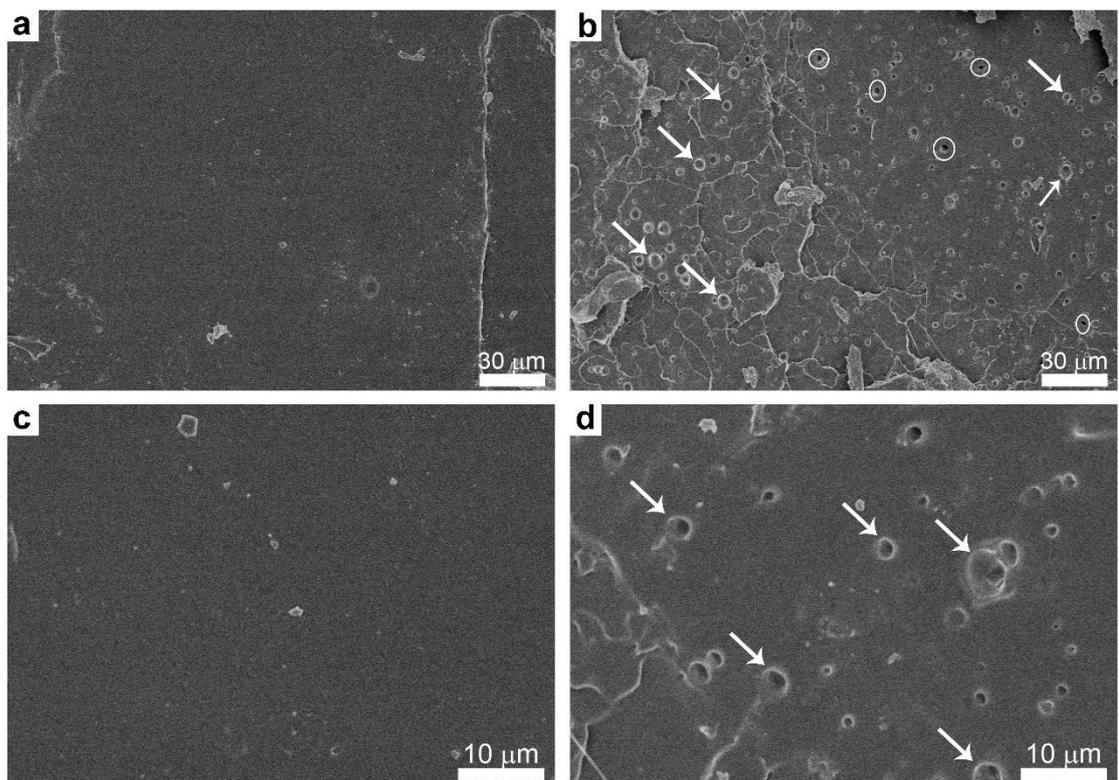
Figure S4. SEM images of cross-section after tensile failure. a, c) PLA, and b, d) PLA/2.0DM-H.
