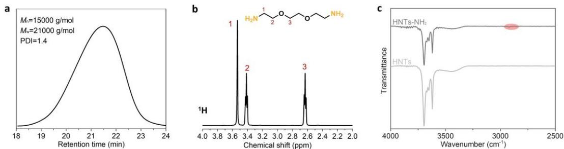
**Figure S1.** Chemical characterization. (a) GPC curve of DM-O, (b)  $^1\text{H}$  NMR spectrum of DADO, (c) FTIR spectra of HNTs and HNTs-NH<sub>2</sub>.
