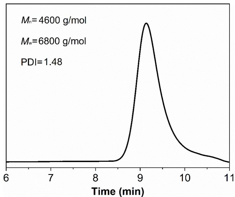
**Figure S1.** The GPC curve of as-synthesized DM-H.
