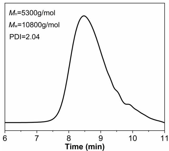
Fig. S1. The GPC curve of DM-Si.
