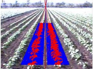
Fig 11. Fitting lines to crop rows
