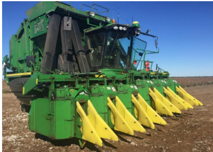
Figure 3.14: The standard John Deere 7760 cotton picker
