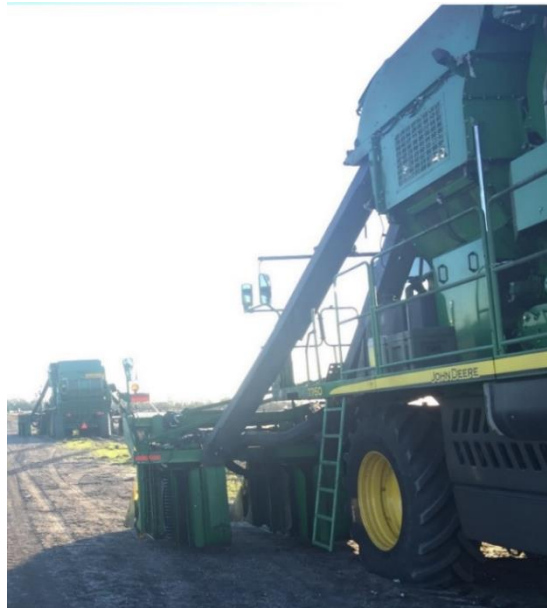
Figure 3.16: A modified the JD7760 cotton picker fitted with single tyres (620/70R42)
