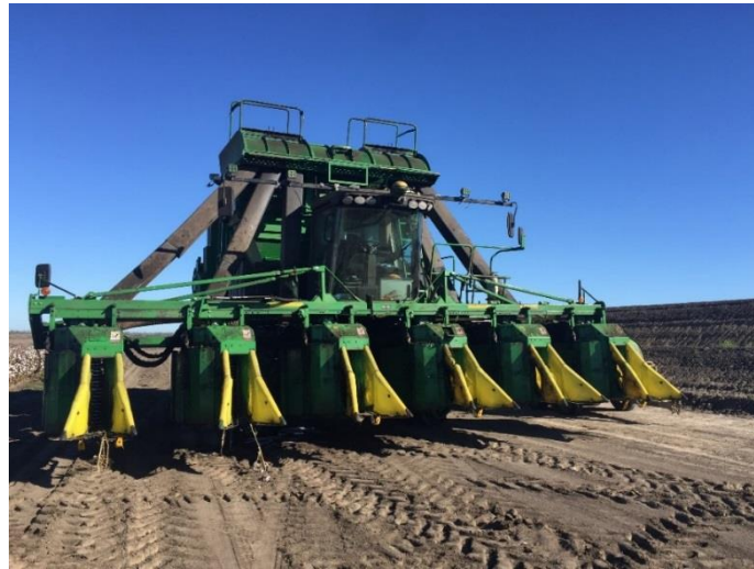
Figure 2.8: The JD7760 modified (9 m frontage with 1.5 m row spacing)
