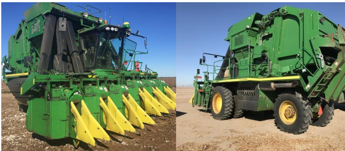
Figure 2.4: The John Deere 7760 cotton picker, noting that the harvester on the right has a front dual-wheel
