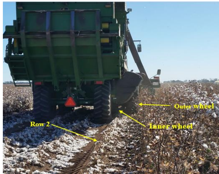
Figure 5.3: Row 2 as influenced by inner and outer dual-wheel traffic of JD7760
