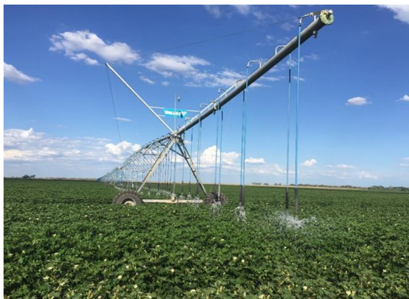
Figure 3.5: Irrigation system of Undabri site (centre pivot system)
