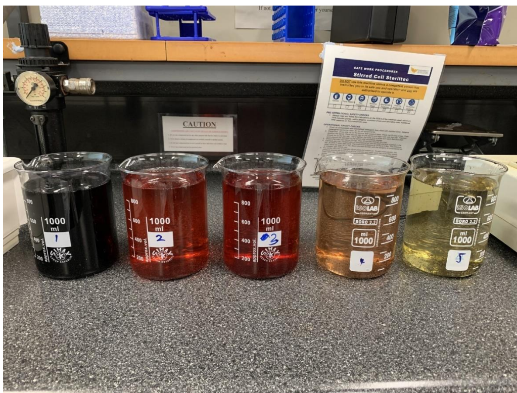
Figure 3. Electrochemical degradation of Reactive Black 5 xenobiotic dye solution after 5 cycles of treatment.
