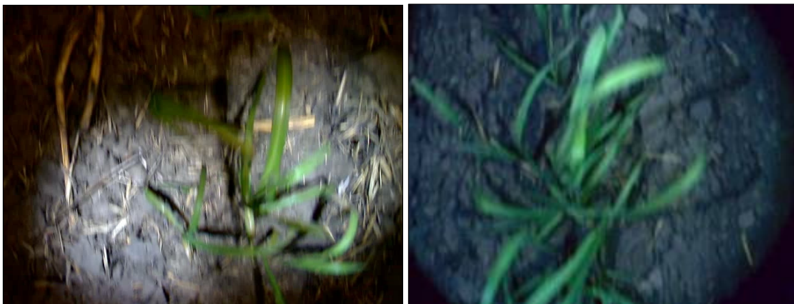
Figure 5. Typical images captured under halogen (left) and LED (right) lighting. The LED lighting appears to illuminate the imaged area more homogeneously.
