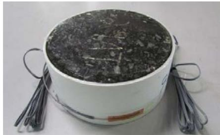
Figure 4.4: Strain gauge set up
