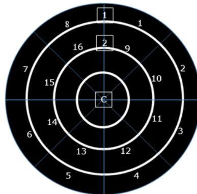
Figure 5.2: 17 transducers locations on each sample for UWT test
