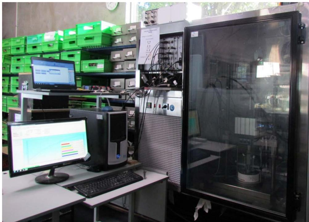
Figure 4.7: Optimisation of UTS tester using an extra data logger
