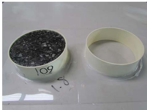
Figure 4.3: PVC confinement set up
