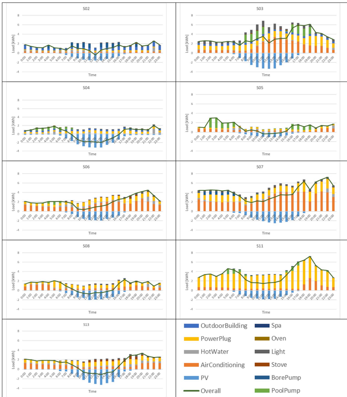
Fig. 1. Daily average patterns of consumption and generation for each circuit type over 3 weeks.
