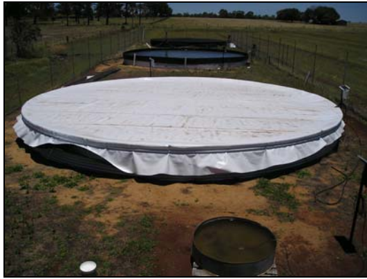
Figure 5-7 Trenched design E-VapCap tied over the edge of the tank.
