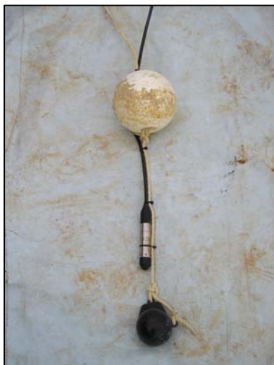
Figure 4-3 Float, rope and sinker used to locate the pressure sensitive transducer out of the silt but in a constant spot.
