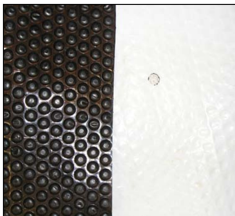
Figure 3-2 E-VapCap has a black side with air filtered bubbles which sit on the water (left hand side) while the white side is exposed to the sun to help reflect incident radiation. Drainage holes in the cover allow rainfall to enter the water storage.
