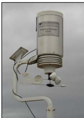
Figure 4-5 WeatherMaster 2000 weather station used to measure the parameters required to run Penman-Monteith.
