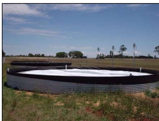
Figure 5-6 Tethered design E-VapCap which floats on the surface of the water but with out being secured to the side of the tank.
