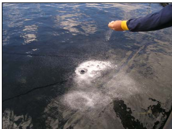
Figure 5-1 Application of monolayer at the USQ Ag plots was repeated at 9:00am every second day during the product's trial.
