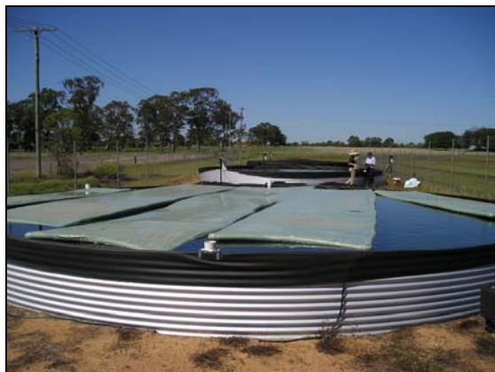
Figure 5-15 The five Raftex modules in the trial tanks at USQ.
