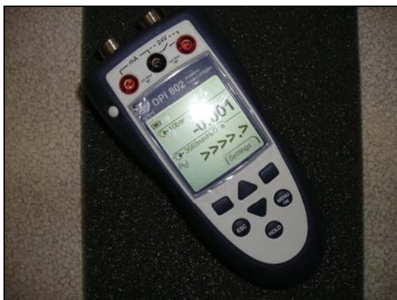
Figure 4-9 Druck DPI 802 portable calibrator used to regularly check the calibration of the Druck PMP 4030 pressure sensitive transducer.
