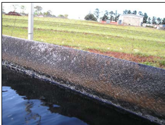
Figure 5-44 The product becomes very sticky and glue like when wetted. This may create problems in field applications.
