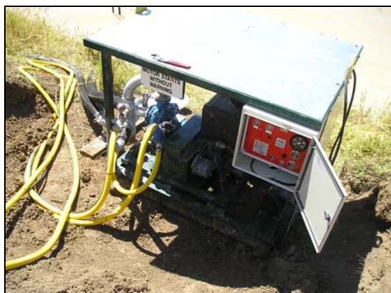
Figure 4-17 Diesel powered pump runs automatically on a timer setup. It has a Murphy system on it to shut down if there are any mechanical problems with the motor.
