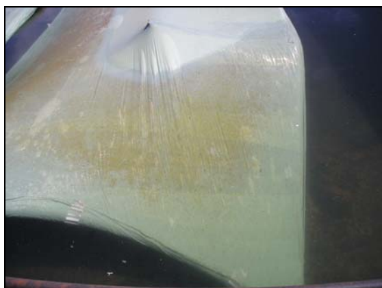
Figure 5-17 Warping or twisting of the Raftex modules as a result of the module being blown off the tank and snapping a wooden cross brace.
