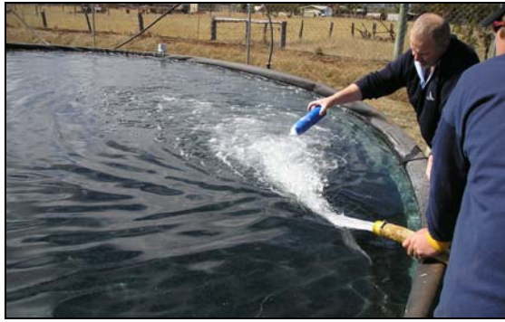
Figure 5-19 Application of PAM was done by hand and the use of a centrifugal pump to circulate the water and distribute the PAM throughout the water body.
