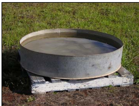
Figure 4-8 Class A pan used at three sites for the comparison with the actual evaporation at St George, Dirranbandi and Toowoomba.
