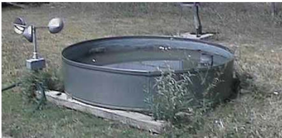
Figure A 2-4 Typical evaporation pan with weeds growing and no bird guard. The pan is also not filled to the top so there will be significant errors associated with the aerodynamics of the lip
