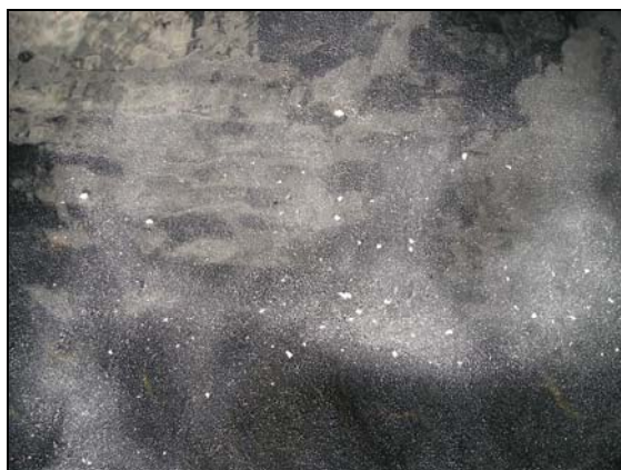
Figure 5-24 Tendency of monolayer to form small beads on top of the water surface when applied by hand.
