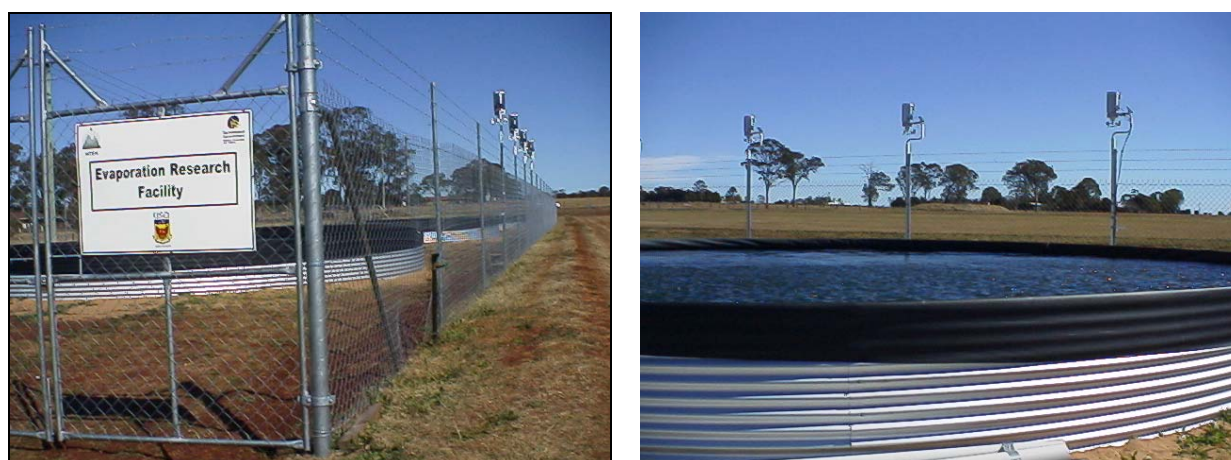
Figure A 2-6 Evaporation research facility based at USQ Ag plot. The experimental trial consists of three lined 10m diameter x 0.8m deep tanks which are being used to accurately assess the effectiveness of different evaporation control methods.
