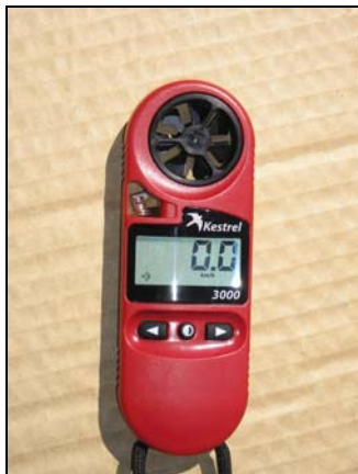
Figure 4-11 Kestrel 3000 is a hand held weather station used to check the calibration of the Envirodata WeatherMaster 2000.
