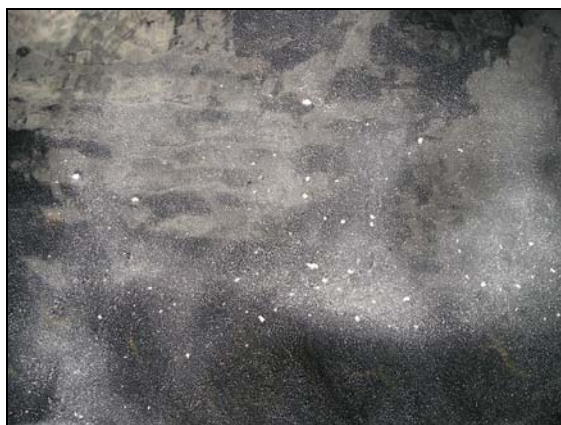
Figure 5-2 Tendency of monolayer to form small beads on top of the water surface when applied by hand.
