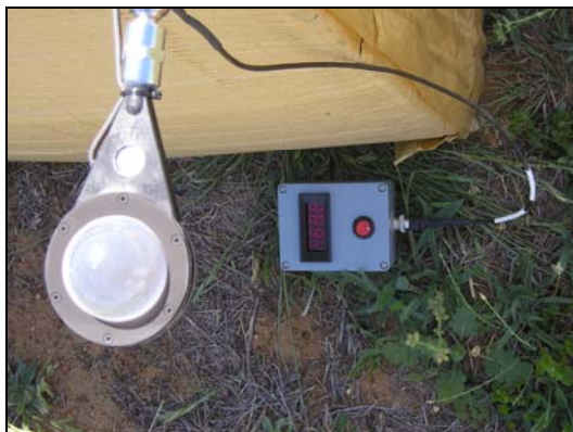
Figure 4-12 Net radiometer from Campbell Scientific used to check the solar radiation on the Envirodata WeatherMaster 2000 weather station.
