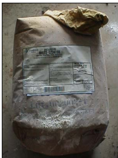
Figure 3-1 The Water$avr product comes in a bag and is applied to the water surface where it spreads itself across the surface creating a thin film to mitigate evaporation.
