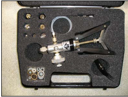
Figure 4-10 Druck PV 211P hand pump used in conjunction with the Druck DPI 802 to apply pressure to the sensors.
