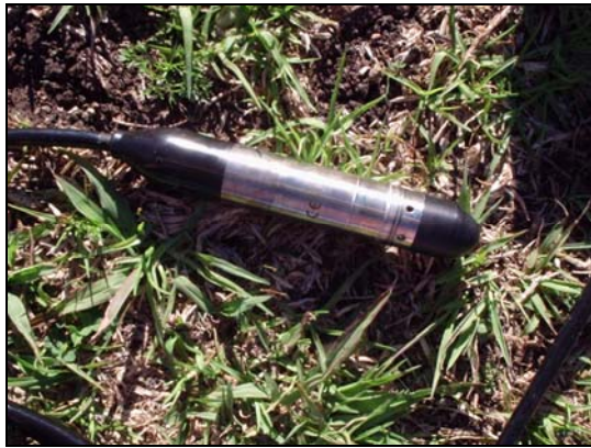
Figure 4-1 Druck PMP 4030 pressure sensitive transducer improved accuracy was used to accurately measure the change in water depth.
