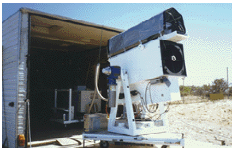
Figure A 2-13 Truck transportable LIDAR machine. The technology uses a scanning UV laser to detect humidity fields and thus deduce total evaporation rates over water bodies.
