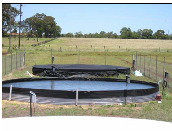
Figure 3-6 Three 10m diameter tanks used to test evaporation mitigation technologies. A maximum of two products were tested at the same time to allow for a control tank to calculate the evaporation saved by the various products.
