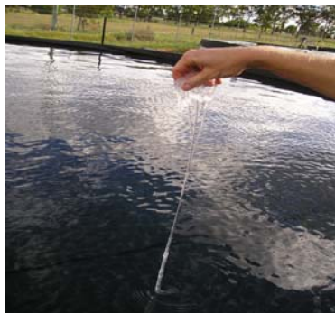
Figure 5-20 Impact of PAM on viscosity of water by binding the water molecules together.
