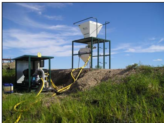
Figure 4-13 Automatic applicator to apply the Water$avr (monolayer) product to a 120ha water storage at Dirranbandi.
