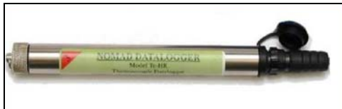
Figure 4-4 Nomad GP-HR general purpose data logger from Intech used to log the depth from the pressure sensitive transducer. The 12 bit logger has three analogue inputs (individually configurable) and one digital pulse input channel.
