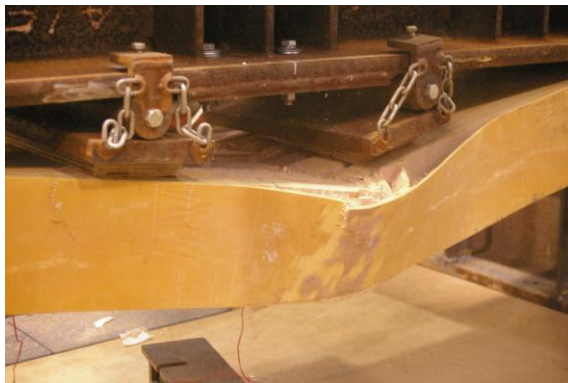
Figure 8.9 Failure of specimen 4F-TS-E
