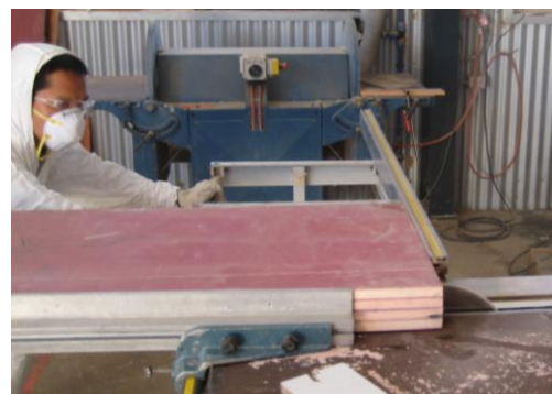
(b) Cutting of sandwich beams
