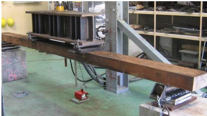
Figure 2.12 Testing of full-size turnout timber sleepers
