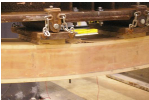
(a) Compressive failure of top skin
