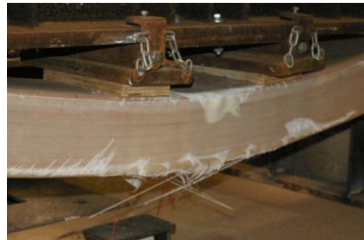
(b) Tensile failure of bottom skin
