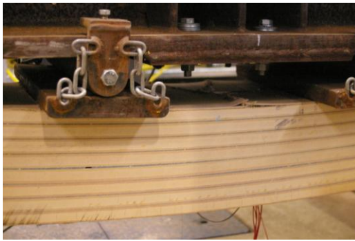
(a) Compressive failure of top skin
