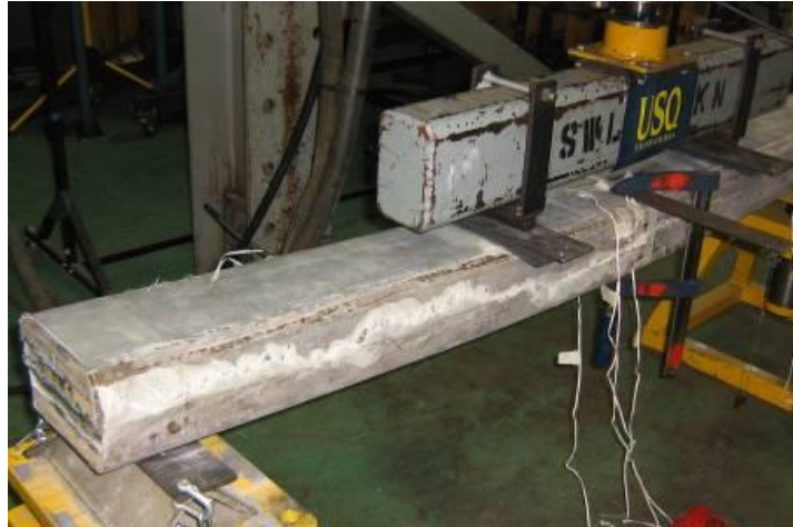
Figure 2.11 Composite sleepers made of LVL wrapped with tri-axial glass fibres
