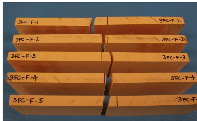
Figure 3.16 Failure of the core under flexural test
