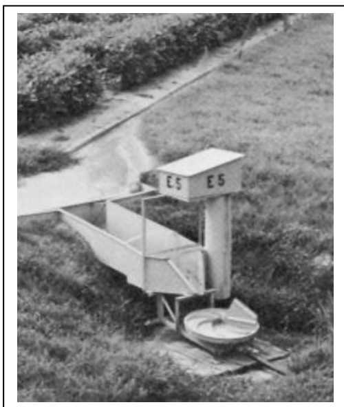
■ Figure 5.4 Flume and Coshocton wheel reproduced from www.rickly.com and accessed on 1 March 2004.
