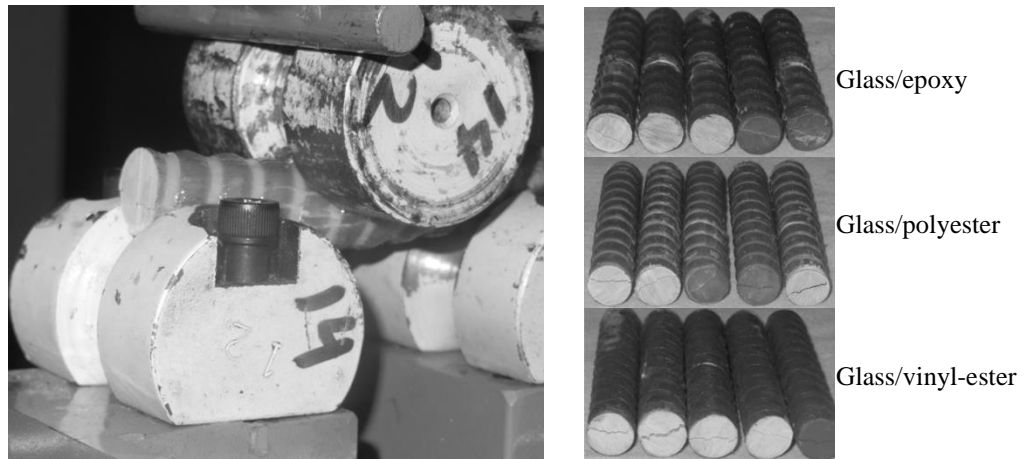
736 Figure 5. Setup for short-beam testing and typical failure mode: (a) test setup; (b) failure mode
