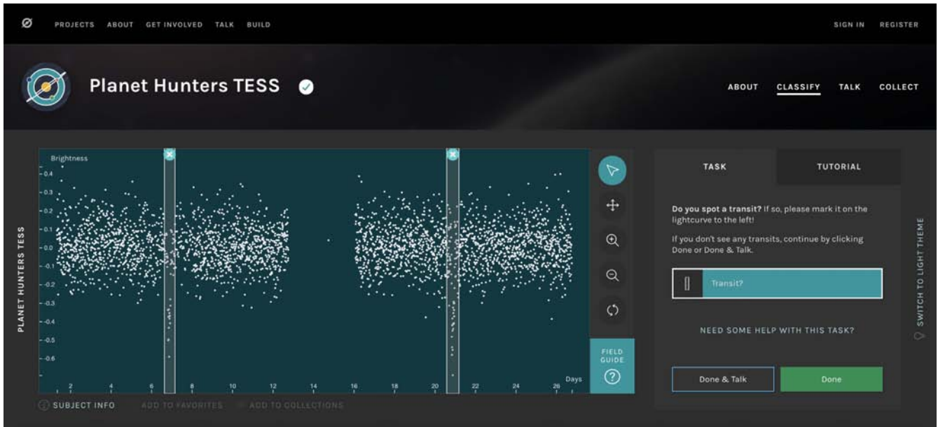
Figure 1. PHT user interface showing a simulated light curve. The transit events are highlighted with white partially transparent columns that are drawn on using the mouse. Stellar information on the target star is available by clicking on ‘subject info’ below the light curve.
