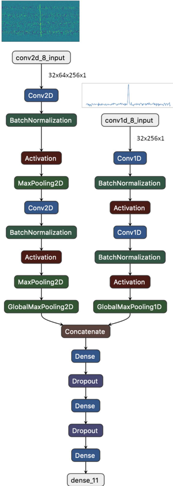
Figure A2. The neural network model architecture of the ML classifier built to identify dedispersed broadband ETI beacons. The model was trained on two different characteristics of the broadband pulse, corresponding to the two branches: the left branch is the spectrogram branch, which takes an input of a 2D dynamic spectrum, while the right branch takes an input of a 1D time series. Both branches were concatenated to assess final probability (see Appendix A.2 for details).
