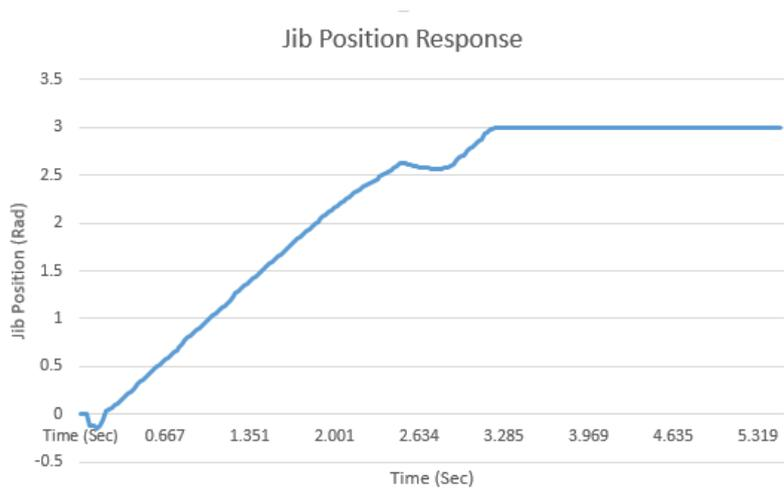
Figure 6-8 Position response of tower jib with no weight
