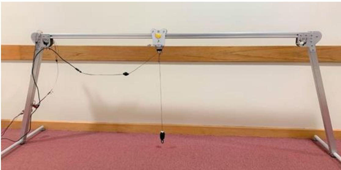
Figure 5-6 The fabricated one axis gantry crane
