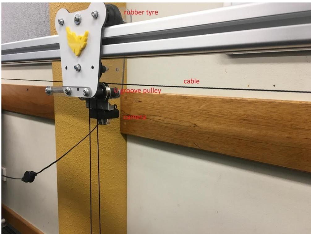
Figure 5-4 The fabricated hoist system
