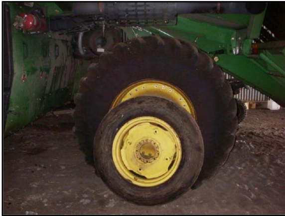
Figure 7 The difference in rear wheel sizes between the JD7760 (back) and a conventional picker (foreground) taken from (McVeigh 2010).
